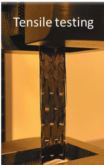
Figure II.3.2.41. Composite specimen tensile testing. Source: Advent.
