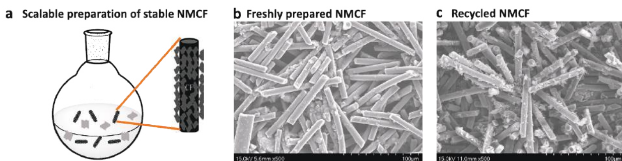
Figure II.3.2.23. (a) Covalent surface functionalization of rCF with carbon nanofiller to form highly stable NMCF. SEM images of (b) freshly prepared NMCF and (c) recycled NMCF from NMVC-R 2 . Due to the strong covalent bonding between CF micro-fillers and carbon-based nanofillers, NMCF is stable even after a series of solution and solid-state processing under heat. Source: RockyTech Ltd.
