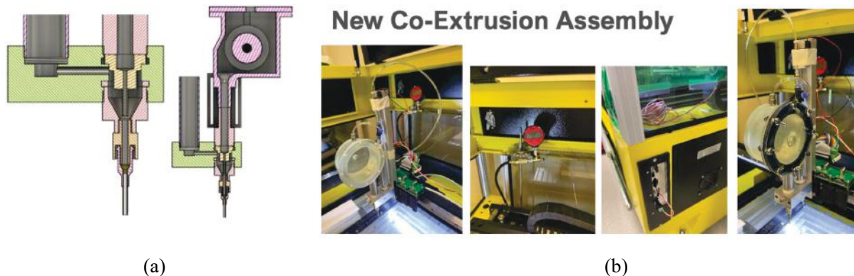
Figure II.3.1.27. (a) 3D-printing of epoxy and continuous CF was initially achieved with the modified Hyrel attachment; however, results were not ideal and backpressure flows are still a problem. (b) A new co-extrusion assembly was designed to have both the fiber and epoxy matrix under the same pressure environment. Source: ORNL.
