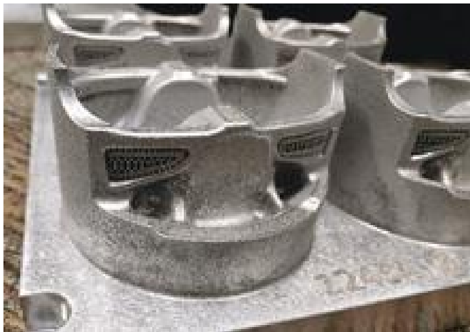
Figure I.2.2.8. AM printed PHASE 2 pistons. Source: ORNL.
