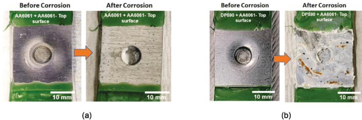
Figure II.4.1.49. (a) Comparison of a representative joint of AA6061 plate joined to AA6061 plate before and after corrosion. (b) Comparison of a representative joint of DP590 plate joined to AA6061 plate (without a rivet) before and after corrosion showing white corrosion product on the surface. Source: PNNL.
