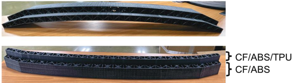
Figure II.3.1.16. Full-scale multimaterial lattice-based bumper. Source: ORNL.
