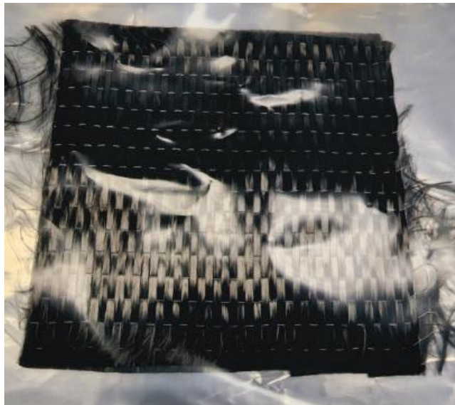
Figure II.3.1.38. CF-PP laminate stack prior to consolidation. Source: ORNL.
