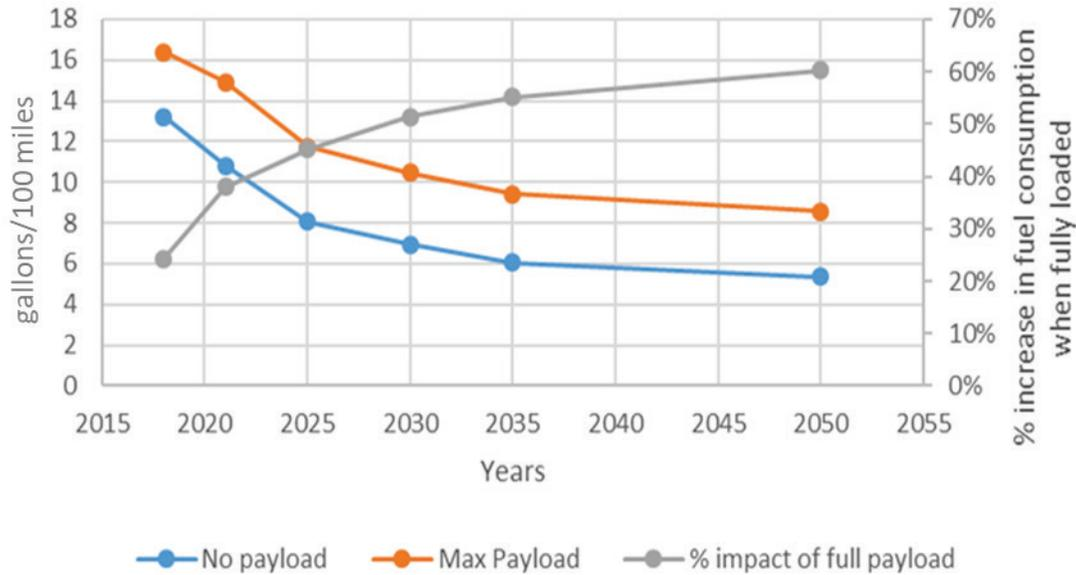
Figure IV.1.3 Impact of different cargo loads on fuel consumption of trucks. Source: ANL
