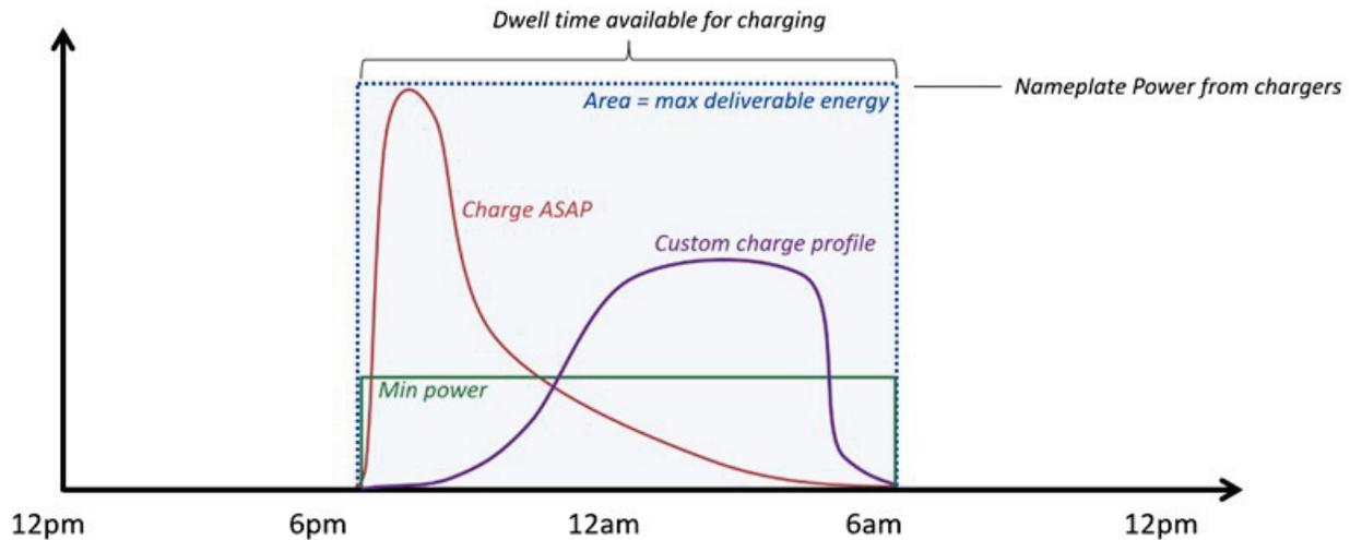
Figure II.3.1 Illustrative example of different charging profiles (charging as soon as possible, charging while minimizing peak power, using a custom charging profile, etc.). Source: EPRI
