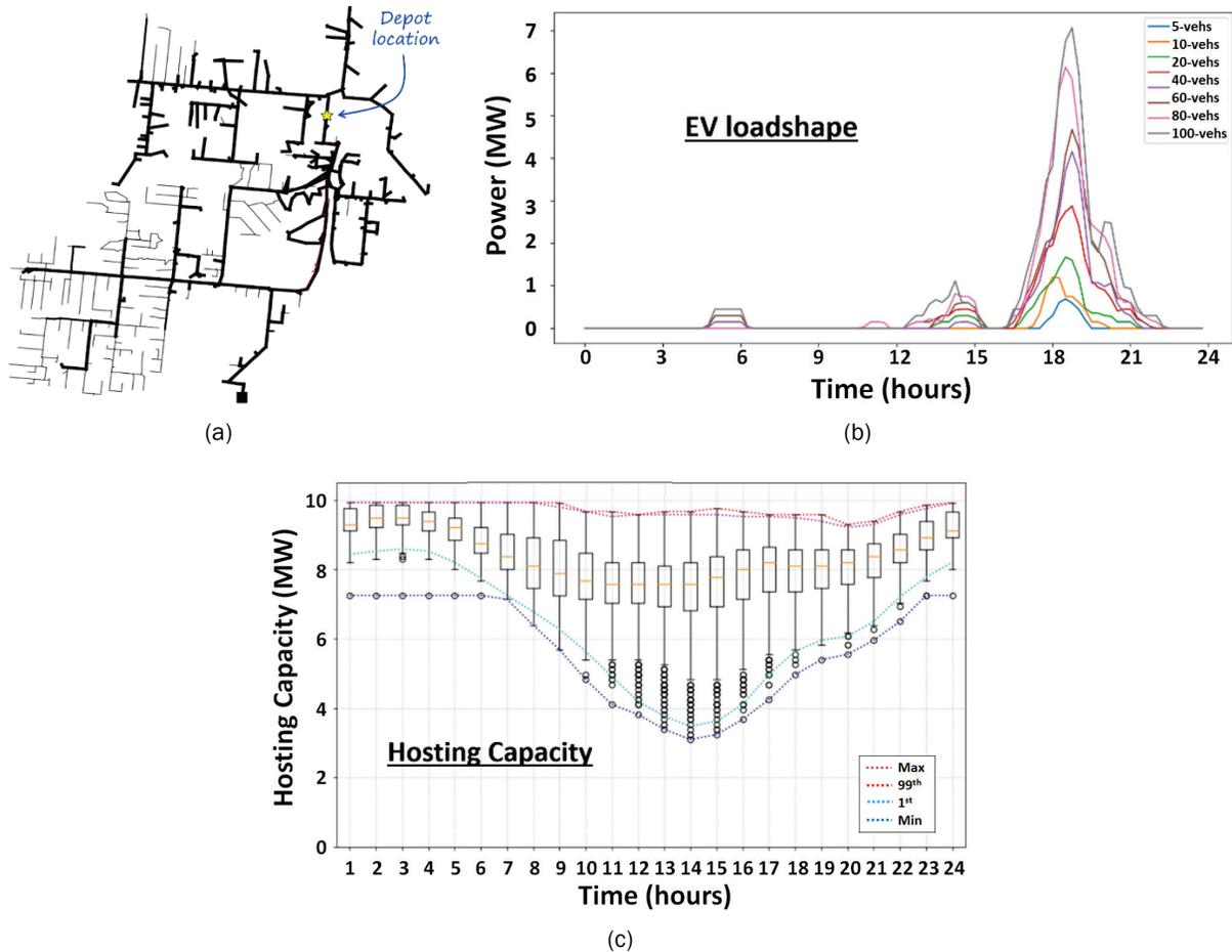
Figure II.3.2 Scenario definition highlighting (a) the assumed depot location, (b) the EV load shapes, and (c) the time-series hosting capacity at that location. Source: EPRI
