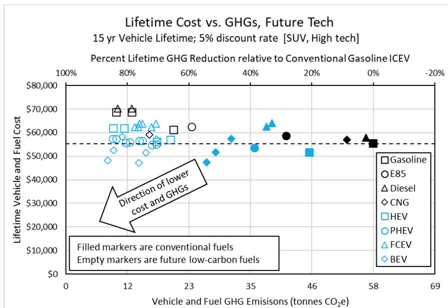
Figure VI.1.3.3 Lifetime cost versus GHG emissions by vehicle-fuel pathway for the FUTURE TECHNOLOGY case for small SUVs (2020\$). Source: Argonne National Laboratory
