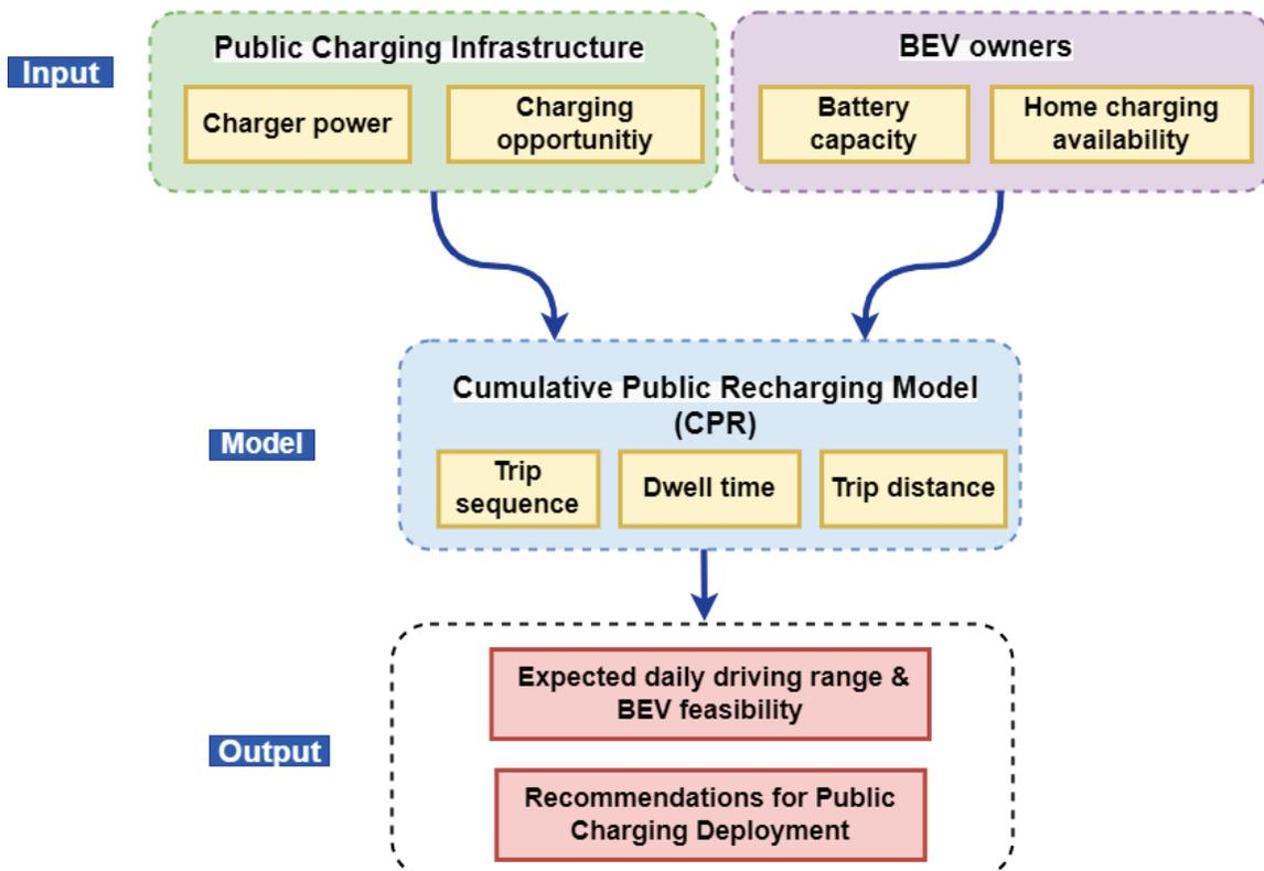
Figure III.1.2 Modeling framework of the Cumulative Public Recharging model used to calculate the expected daily driving range and BEV feasibility as well as recommendations for public charging deployment. Source: ORNL
