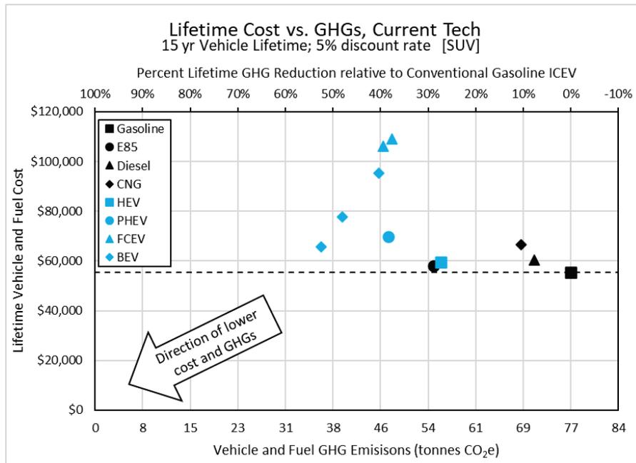
Figure VI.1.3.2 Lifetime costs versus GHG emissions by vehicle-fuel pathway for the CURRENT TECHNOLOGY case for small SUVs (2020\$). Source: Argonne National Laboratory
