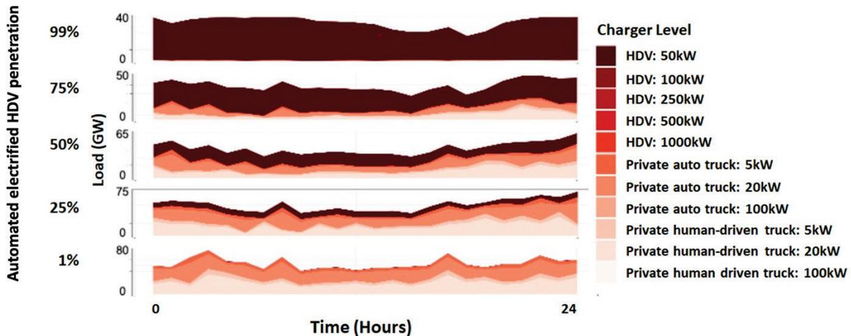
Figure II.1.2 Electrified HDV daily charging load profiles across scenarios of electric and automated vehicle (EV/AV) penetration. Source: Lawrence Berkeley National Laboratory
