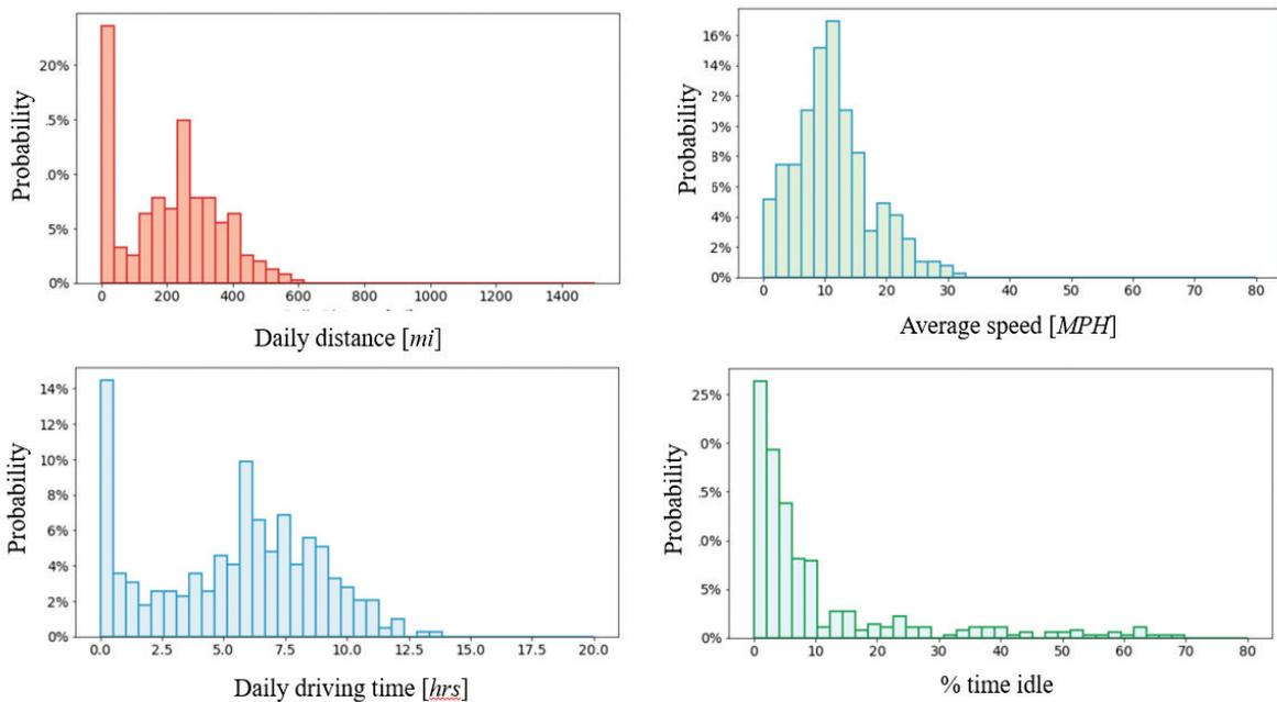
Figure II.5.2 Aggregated vehicle statistics using a cloud-connected service trip summary table. Source: University of Minnesota
