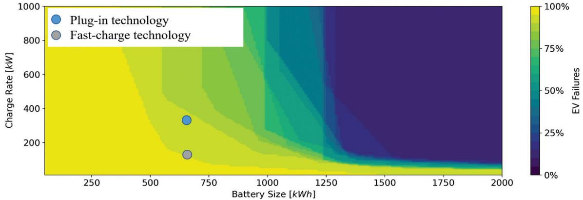
Figure II.5.3 Battery estimates with respective EV failure rates. Source: University of Minnesota
