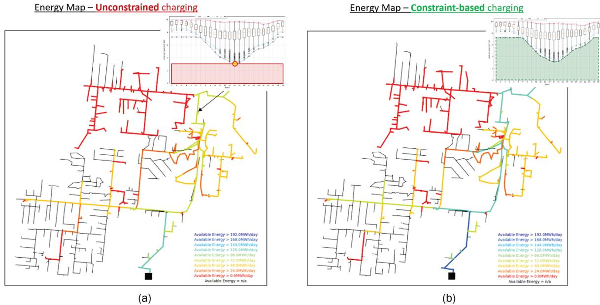
Figure II.3.5. Energy availability at different locations on a distribution feeder under two types of charging strategies: (a) unconstrained and (b) constraint-based. Source: EPRI
