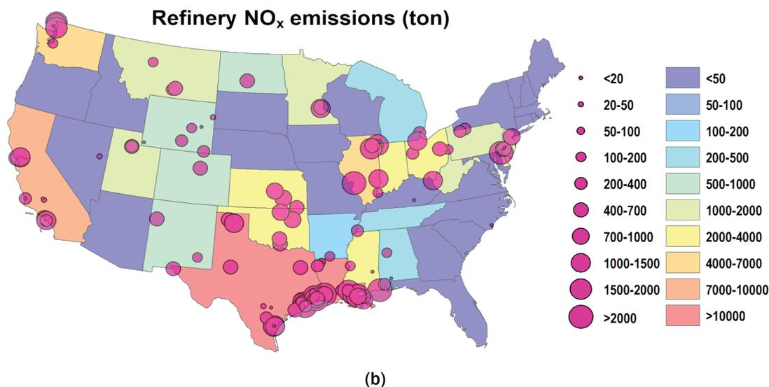
Figure VI.1.2.1 (a) NO<sub>x</sub> emissions from power plants and (b) petroleum refineries in the United States. The size of circles indicates the facility emissions, and the color of states demonstrates the state emissions. Source: Argonne National Laboratory
