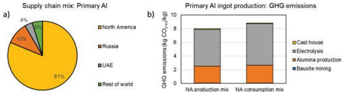
Figure VI.1.1.1 (a) Share of different sources in total primary Al supply to North America (based on [7]); and (b) GHG burdens of primary Al ingot based on GREET simulation (NA production mix: primary Al production in North America; NA consumption mix: primary Al consumed in North America). Source: Argonne National Laboratory
