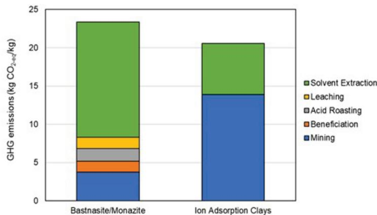
Figure VI.1.1.4 GHG emissions for REO production from different ore types (based on GREET simulation). Source: Argonne National Laboratory
