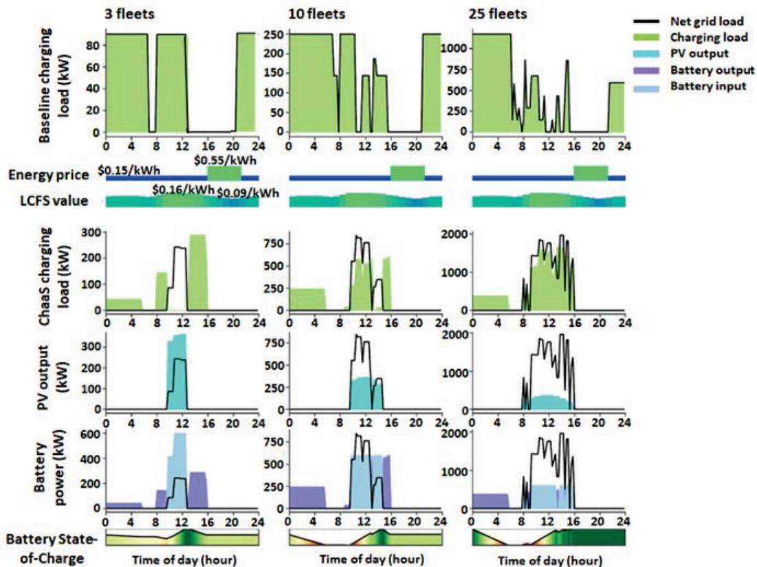
Figure III.4.1 Baseline charging comparison with CaaS, PV output, battery power and the battery state-of-charge. Source: Colorado State University
