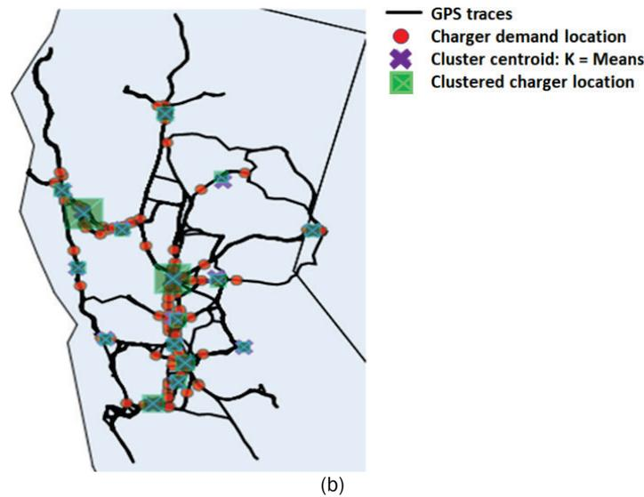
Figure II.5.7 (a) Capital expenditure analysis with various clustering methods and (b) charging stations for k-means clustering of 16 clusters. Source: University of Minnesota
