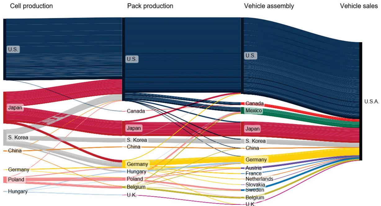
Figure I.2.2 Sankey flow diagram showing manufacturing locations for cells, packs, and vehicles for PEVs sold in the United States from 2010 to 2021 (in terms of total battery capacity in gigawatt-hours). Source: Argonne
