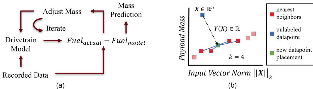
Figure II.5.4 (a) Model-based mass estimation and (b) data-driven mass estimation. Source: University of Minnesota
