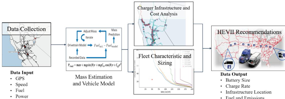
Figure II.5.1 Depiction of the HEVII tool stages: data input, analysis, and resulting data output. Source: University of Minnesota
