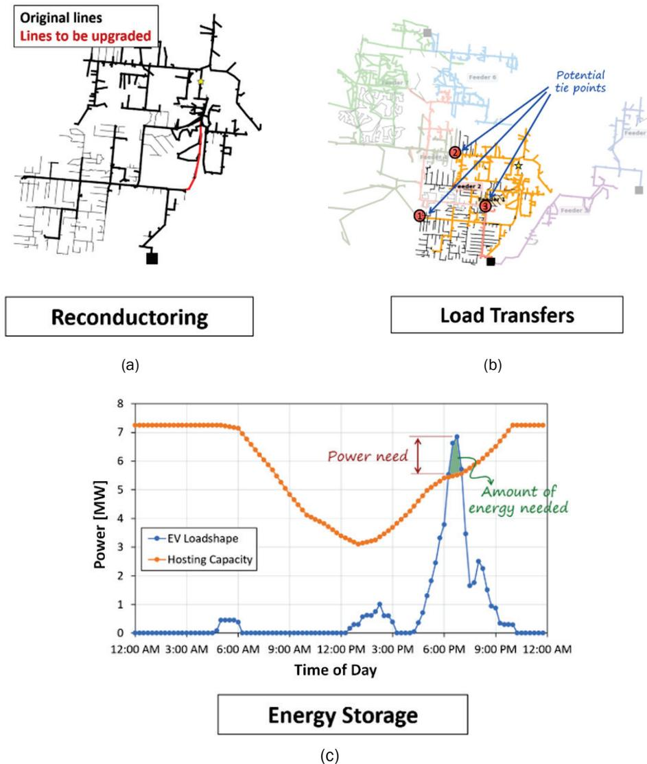
Figure II.3.3 Mitigation solutions to accommodate fleet electrification on distribution feeders for (a) reconductoring, (b) load transfers, and (c) energy storage. Source: EPRI
