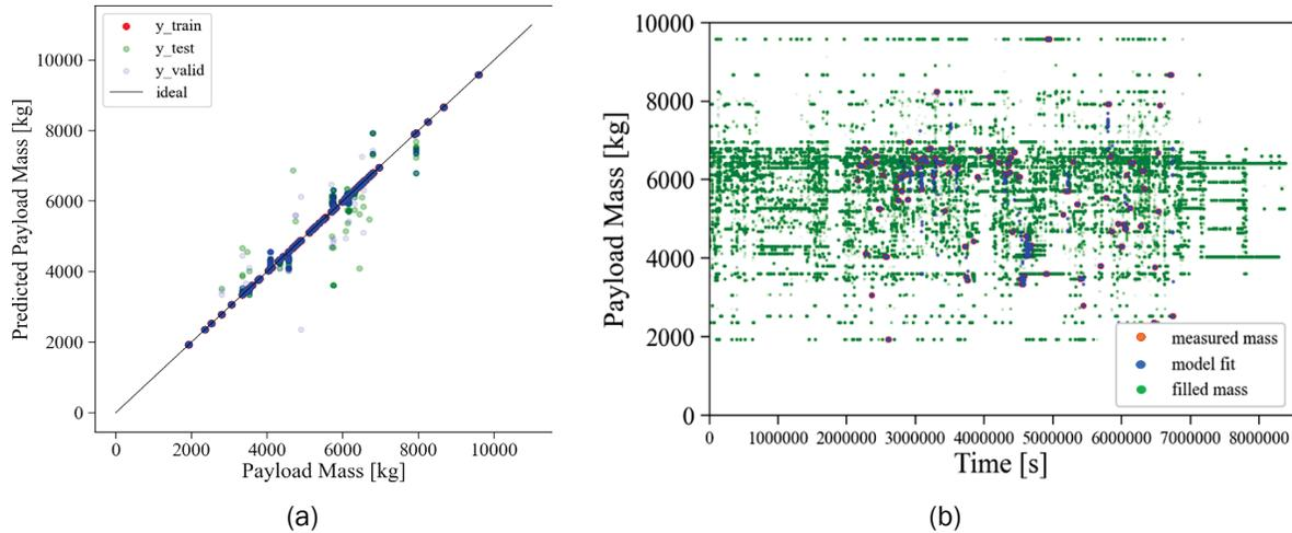
Figure II.5.5 (a) Results after fitting kNN regressor and (b) the predicted mass history. Source: University of Minnesota and NREL
