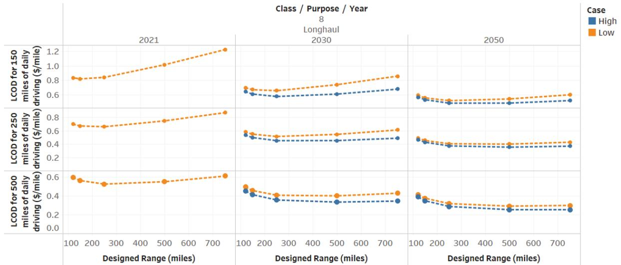
Figure IV.1.5 Impact in cost of driving for different designed BEV ranges across different miles of daily driving, including a dwell time penalty of \$75/hour. Source: ANL
