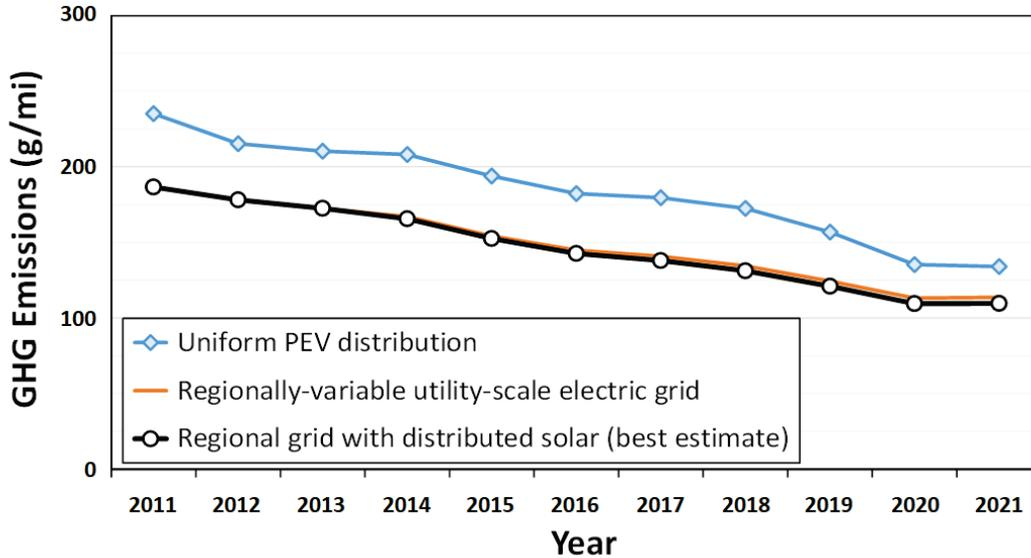
Figure I.2.1 Comparison of average well-to-wheels GHG emissions weighting for all registered PEVs in the United States from 2011 to 2021. The blue line represents a uniform national distribution of vehicles and electricity generation, the orange line accounts for the spatial distribution of vehicle registrations, and the black line includes the impacts of distributed solar generation. Source: Argonne
