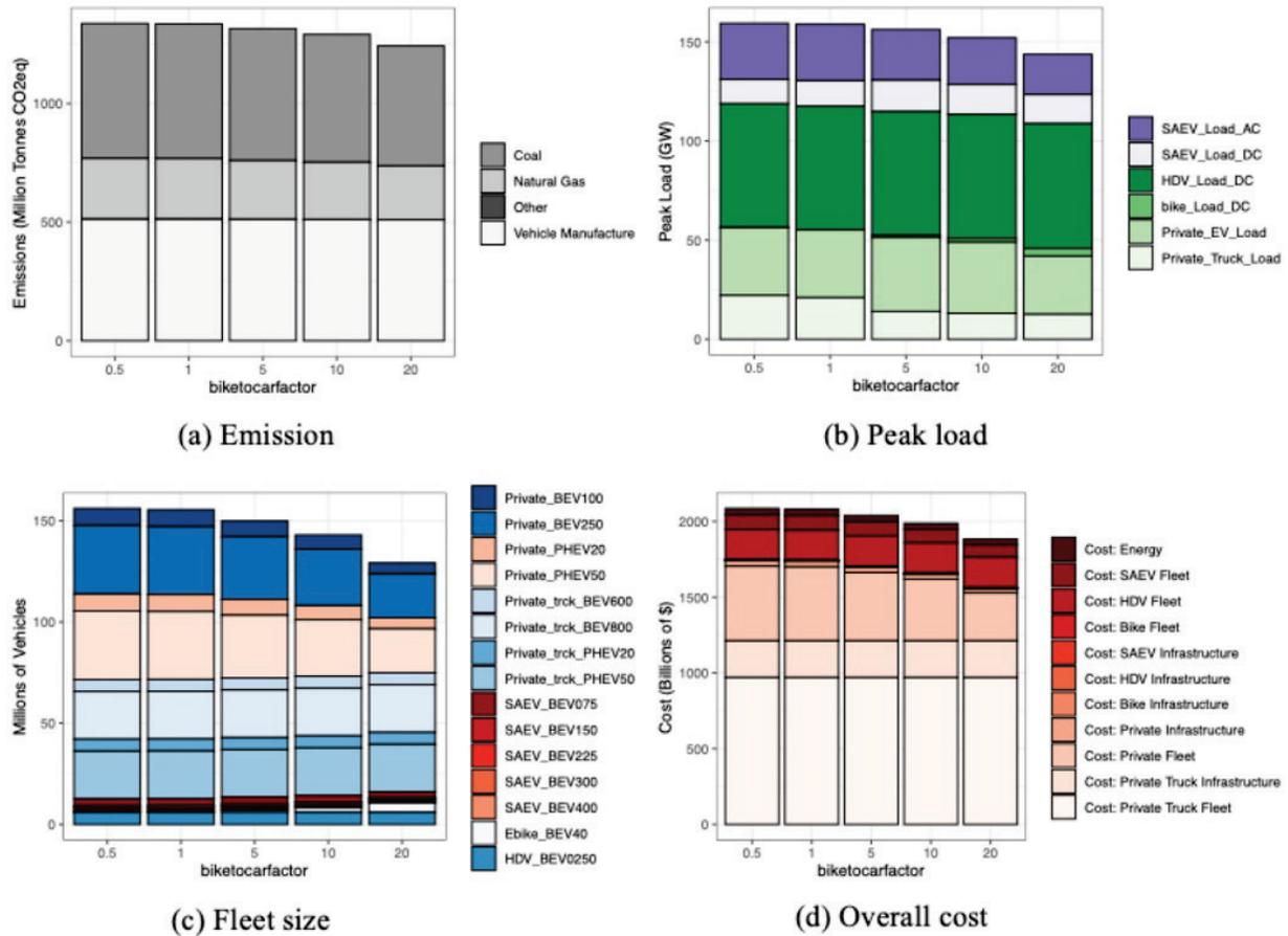
Figure II.1.4 Penetration of electrified micro-mobility panel showing increases in the fraction of bike-to-car trips and associated changes in (a) GHG emissions, (b) peak power demand, (c) fleet sizes, and (d) overall costs. Source: Lawrence Berkeley National Laboratory
