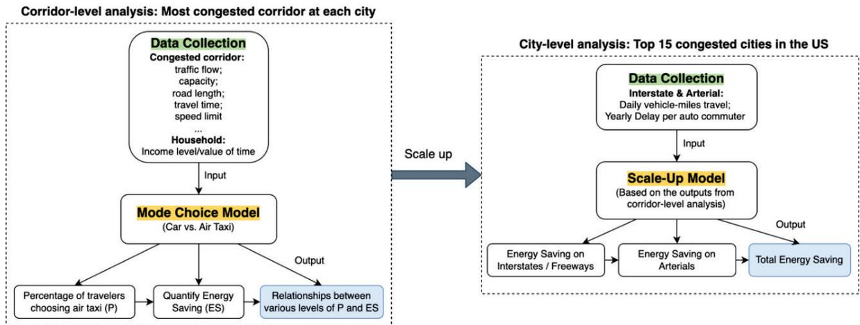
Figure III.1.3 Modeling framework used to extend and scale up the previous corridor-level model and to quantify the nationwide impact of air taxis on driver travel time and on-road energy use. Source: ORNL
