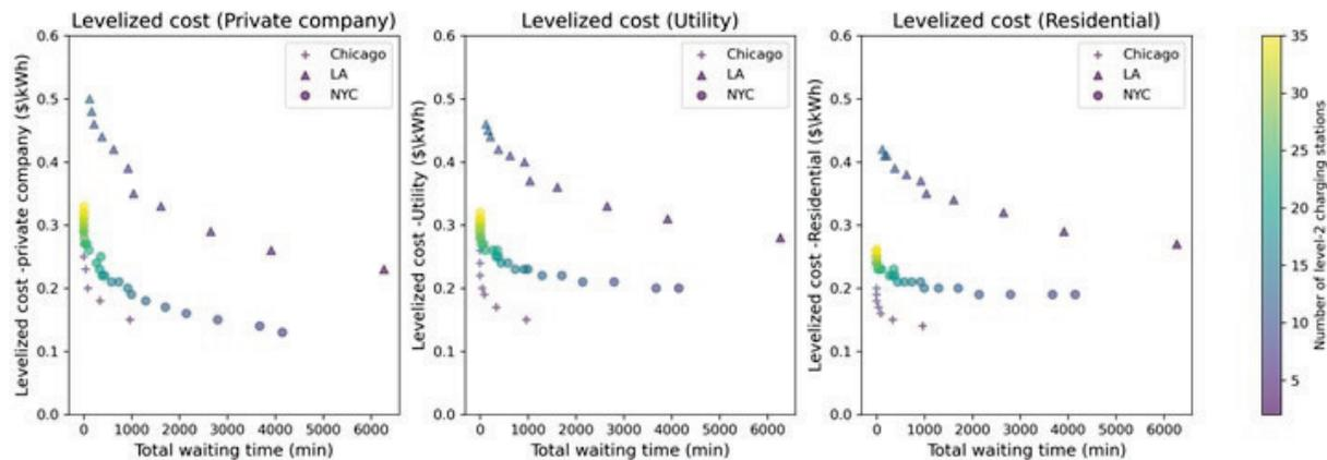
Figure II.4.3 Trade-offs between levelized cost of charging and total waiting time, when only Level 2 charging stations are installed in the MUD charging hub. Source: UIUC
