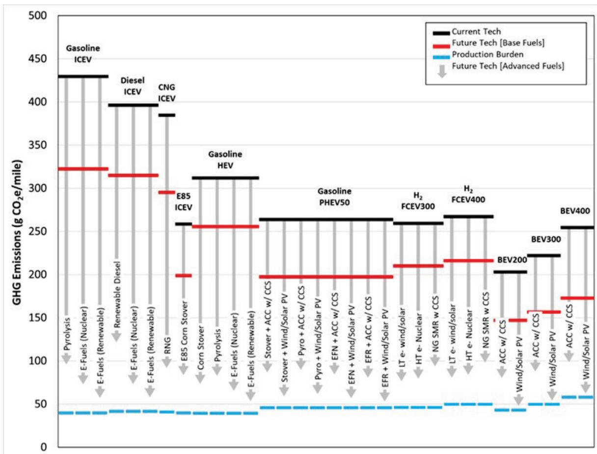
Figure VI.1.3.1 C2G GHG emissions of various vehicle-fuel pathways for small SUVs assuming high technology progress. Analysis was performed using GREET2020. Source: Argonne National Laboratory
