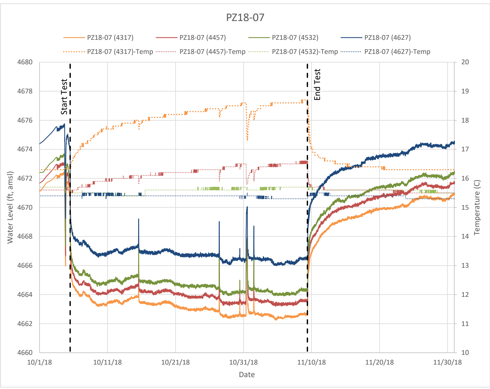
PZ18-07 Water level and Temperature Hydrograph
