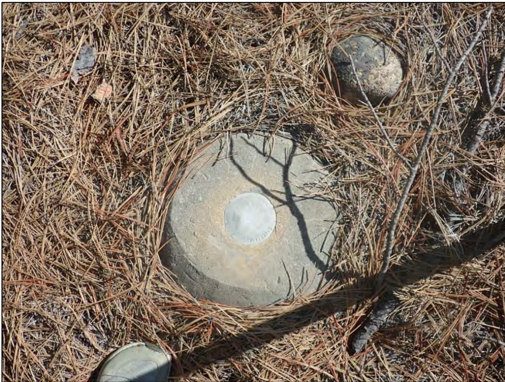
PL-4. Combined Survey and Boundary Monument 1
