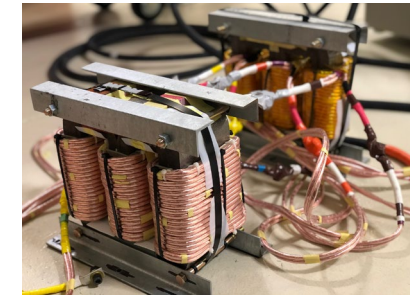
75 kVA Configuration Inverter Inductor Power Testing
