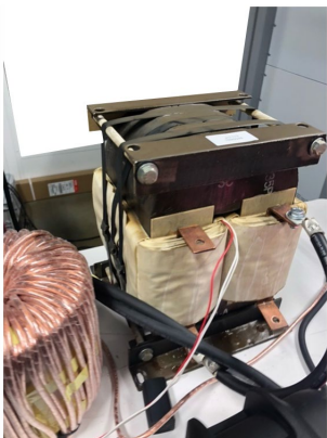
Multigap smoothing inductor 1mH, 1 kHz, six gaps
