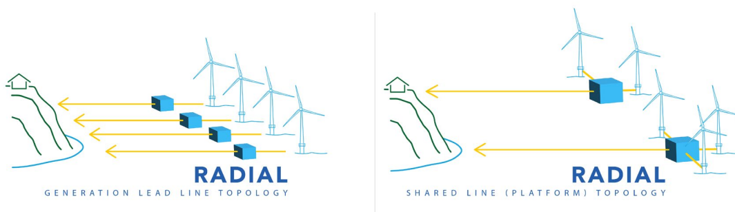
Figure 7. Radial transmission topologies (offshore wind plants represented as single turbines).
