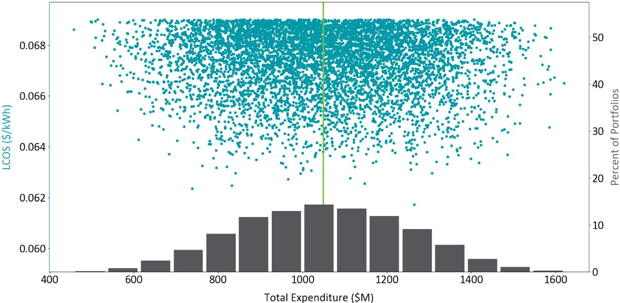
**Figure 4. LCOS and expenditures for the top 10% of portfolios for LIBs. The axis on the left labels the scatterplot of expected LCOS for each portfolio versus total expenditure, while the axis on the right labels the histogram of expenditures. This means that the histogram shows the distribution of the dots on the scatterplot. The vertical line marks the median expenditure.**
