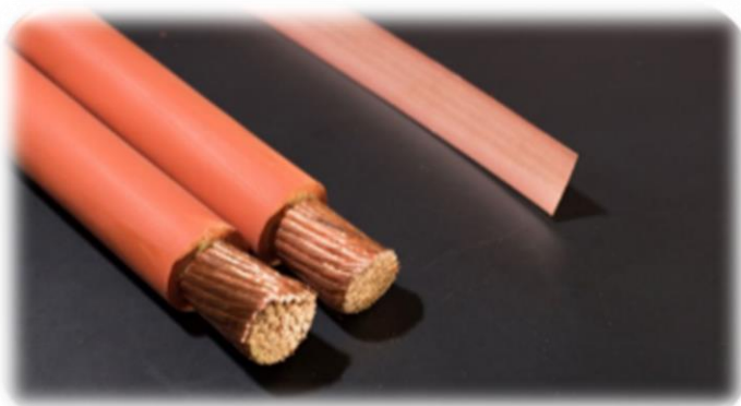
Figure 10: Visual Size Comparison of REBCO tape superconductor and Copper capable of carrying equivalent current. (Selvamanickam 2022)
