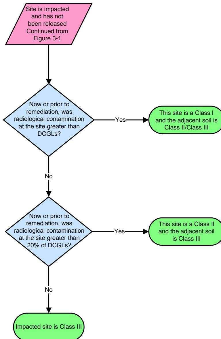
Figure 3-3. Process to Determine Remaining Activities – Adjacent Soil
