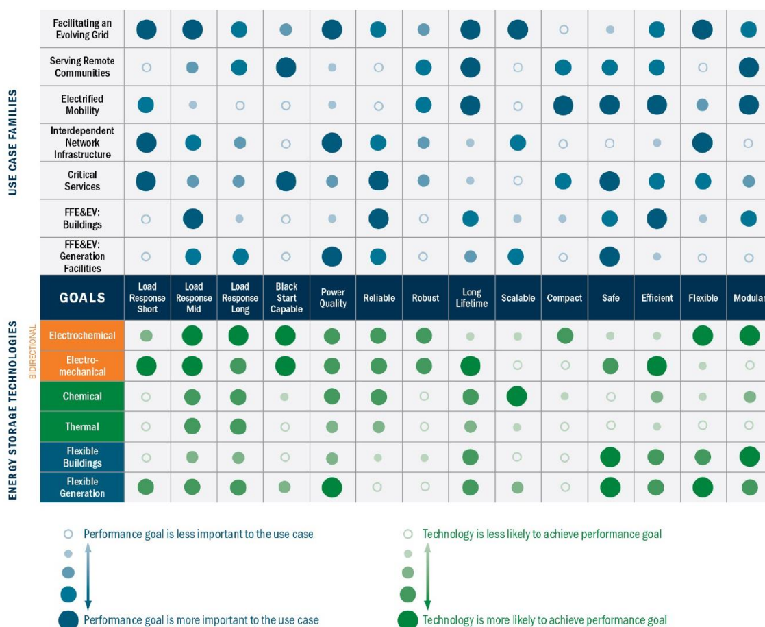
Figure 6.2: Performance characteristics (green circles) and applicability to use cases (blue circles) of multiple classes of energy storage technologies. Figure reproduced from DOE's Energy Storage Grand Challenge Roadmap (2020). (FFE&EV = Facility Flexibility, Efficiency, and Enhanced Value)
