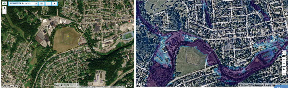
(a) (b) Figure 16. Canonsburg, PA: (a) the site boundary from the GEMS database and (b) the flooding extent from the First Street Foundation Flood Model. In (b), the light blue area is the flooding extent up to the depth of 1 meter, while the purple area is the one of larger than 1 meter.
