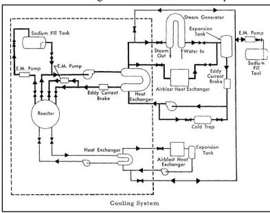
heat from the primary sodium to a secondary loop which in turn dissipated the heat to the atmosphere via an airblast heat exchanger. The second option, shown in the upper portion of the figure, transferred the heat from the primary sodium to a secondary sodium loop which in turn dissipated the heat in a steam generator that boiled water to make steam for use in a turbine/generator that produced electricity for the Southern California Edison grid.<sup>3</sup>
