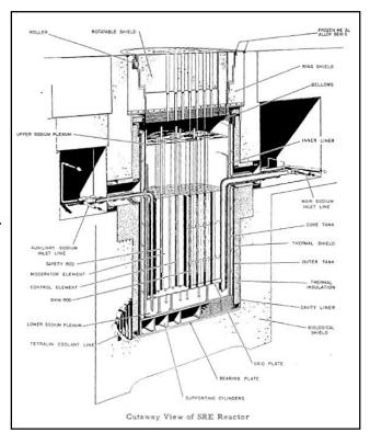
Piping circulated 50,000 pounds of heated liquid sodium from the reactor vessel to either of two available heat exchangers. As shown in the lower portion of the figure, one option transferred the
