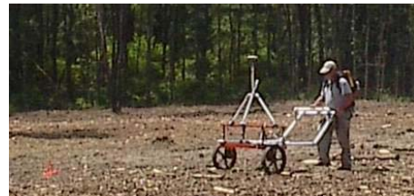
Figure 2: Example of an EM61 coupled with a Leica 1200 DGPS.
