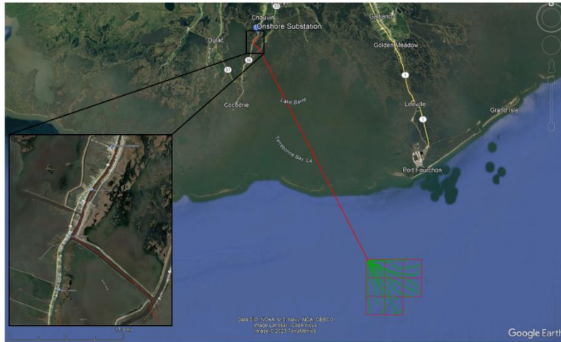
Figure 5. Export cable route from offshore substation to point of interconnection and export cable landfall in Chauvin, Louisiana.
