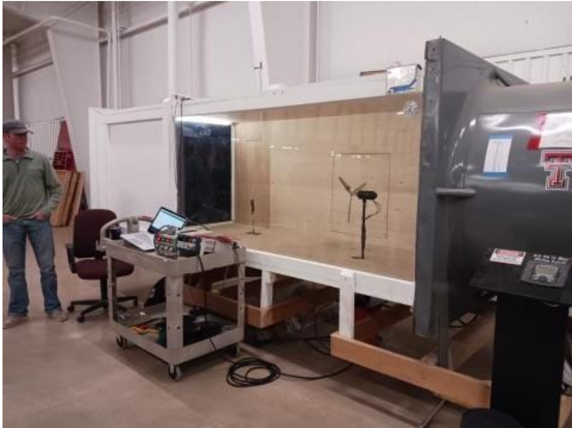
Figure 2: 1.2 m x 1.2 m wind tunnel at Reese Technology Center.
