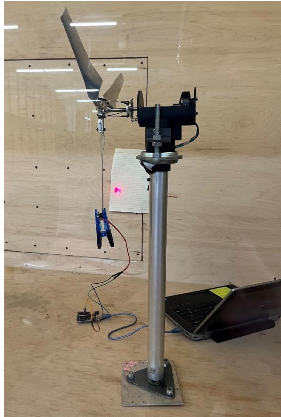
Figure 4: Rotor pitch laser calibration.
