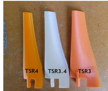
Figure 3. Blade geometries by TSR
