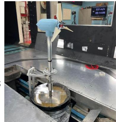
Figure 28. Fully-assembled turbine with offshore tank
