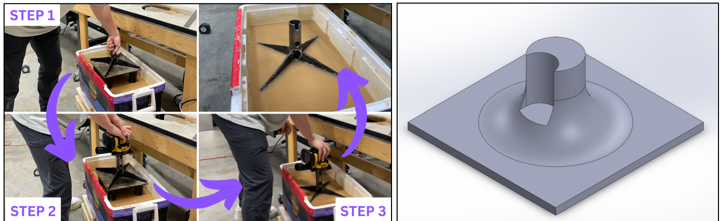
Figure 13: Installation Process and Sander Tool with 3D Printed Adapter Piece
