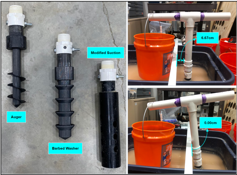
Figure 9: 3D Printed Anchoring Pile Design Prototypes and Test Setup
