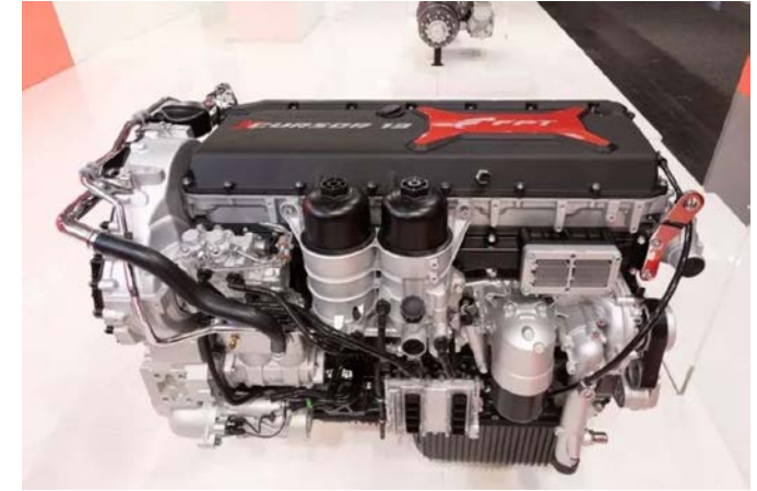
FPT XC13 13L multi-fuel engine
