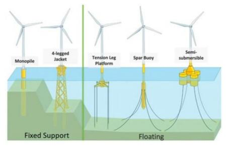
Figure 2.6. Support structures for offshore wind turbines (NREL, 2020).
