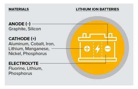
Figure 2.2. Materials used in lithium-ion battery components.
