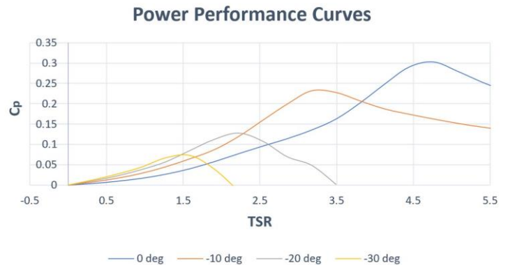
Figure 2.2.2: Power Performance Curves
