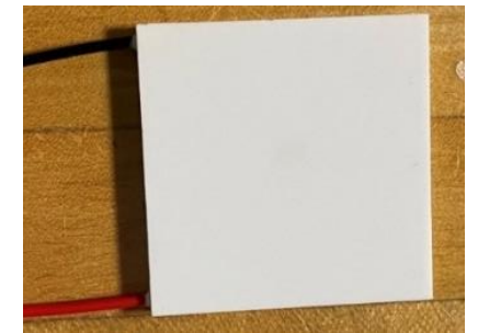
Pi-type ( \pi ) commercialized TE module 4 $/piece (60 W)
