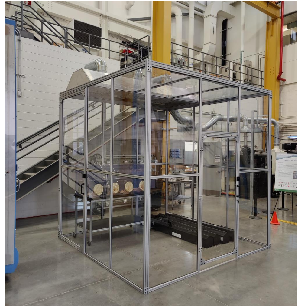
Ventilation enclosure with exhaust air to allow safe spraying in the lab
