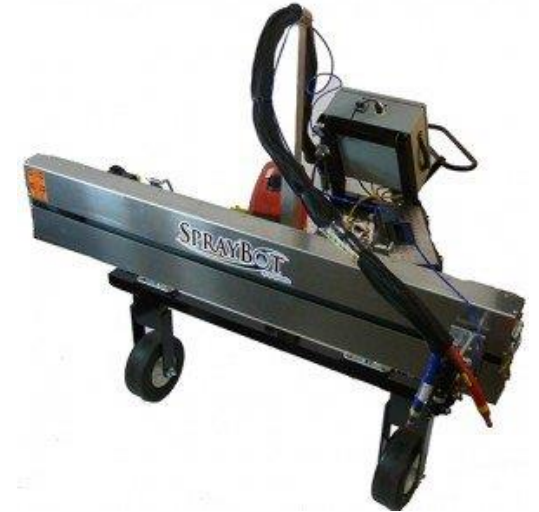
SprayBot for roof SPF install by SprayWorks
