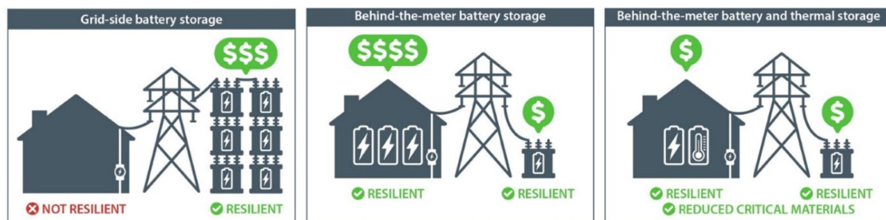
Figure 2. Three scenarios for future national-scale energy storage. (Left: Using only electricity-to-electricity (E-to-E), the grid side will require a very large investment. Middle: Moving E-to-E storage behind the meter will increase the cost but provide additional resilience to buildings. Right: Using thermal storage in buildings with E-to-E both in front and behind the meter may offer a pathway with the lowest overall cost to society.)
