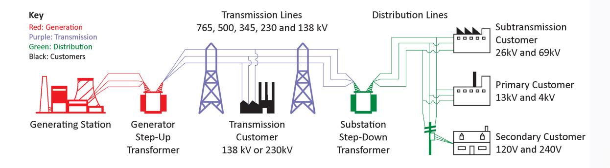
Note: 161 and 115 kV Transmission Voltages Exist Note: 46, 34.5, 23 kV and other Distribution Voltages Exist
