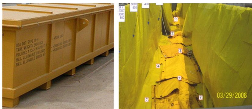
Figure 2. Exterior of B-36 Disposal Container (Left) and Actual Tank 28F Salt Sampling Drill String and Lead Blankets in B-36 Disposal Container (Right).
