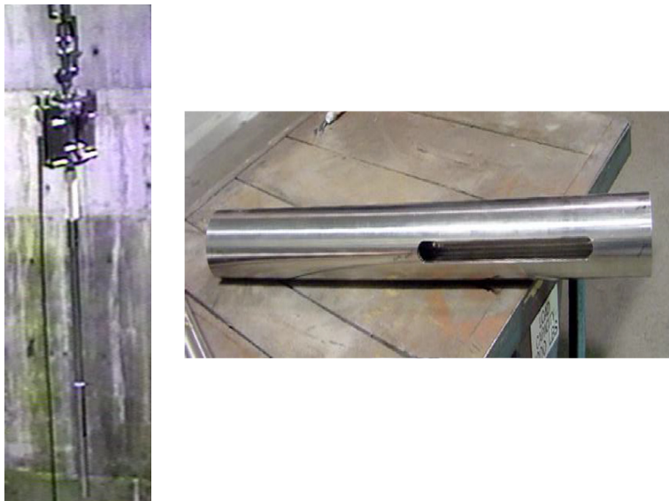
Figure 4. Glass Pump (close-up of Inconel pipe on right).
