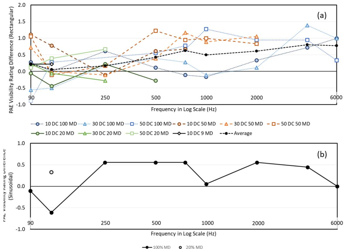
**Figure 14 (a, b). Differences between higher and lower sensitivity participant phantom array effect (PAE) visibility ratings for rectangular waveforms (a) and sinusoidal waveforms (b).**
