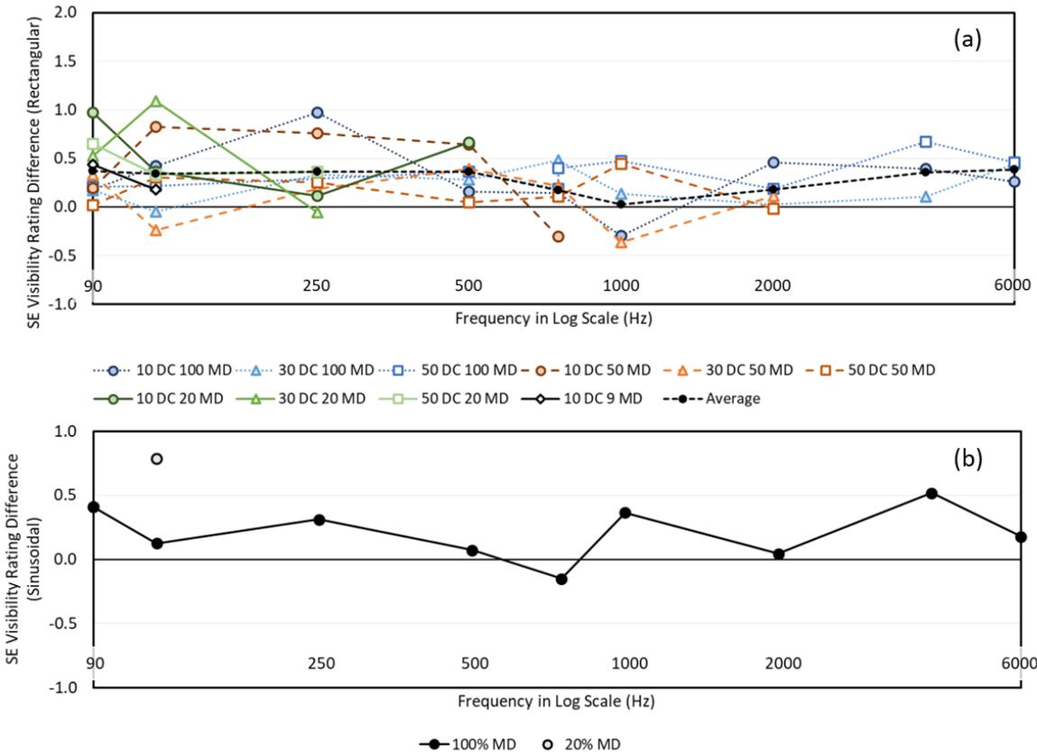
**Figure 15 (a, b). Differences between higher and lower sensitivity participant stroboscopic effect (SE) visibility ratings for rectangular waveforms (a) and sinusoidal waveforms (b).**
