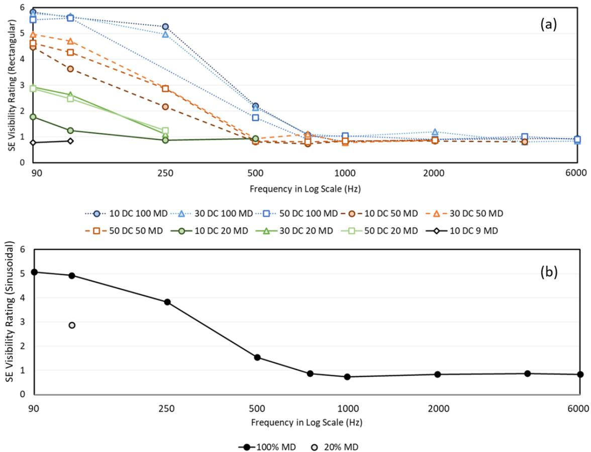
**Figure 9 (a, b).** Plot of arithmetic average participant stroboscopic effect (SE) visibility ratings for 30 observers for all 61 rectangular TLM waveforms (a) and all 10 sinusoidal TLM waveforms (b).
