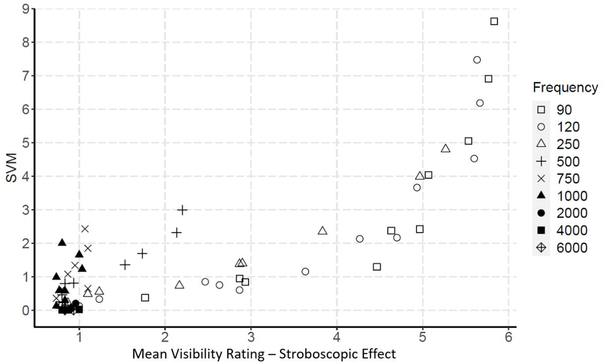
Figure 18. Mean stroboscopic effect visibility ratings plotted against SVM for each TLM waveform.
