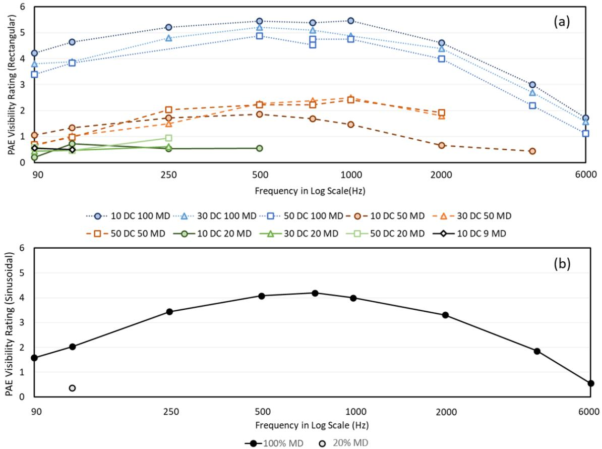
**Figure 7 (a, b). Phantom array effect (PAE) visibility: Arithmetic average ratings for rectangular waveforms of different frequency, modulation depth (MD), and duty cycle (DC) (a); and sinusoidal waveforms of different frequencies (b).**
