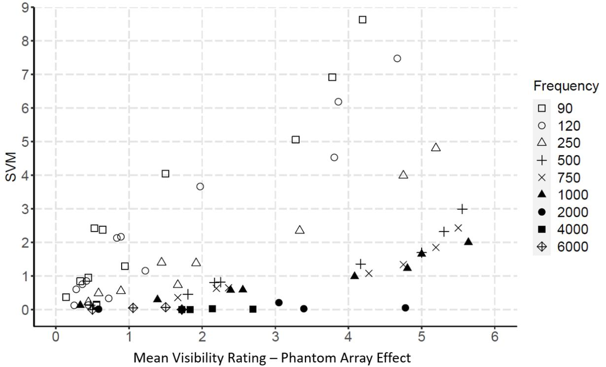
Figure 17. Mean phantom array visibility ratings plotted against SVM values for each TLM waveform.
