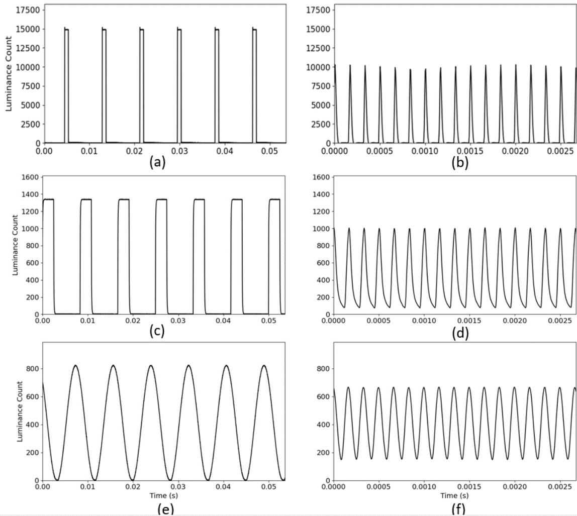
**Figure 3 (a – f).** Plots (a), (c), and (e) illustrate the output of three 120 Hz, 100% modulation waveforms, rectangular with 10% duty cycle in (a), 30% duty cycle in (c), and a recognizable sine wave in (e). Plots (b), (d), and (f) illustrate the output of three 6,000 Hz, 100% modulation waveforms, “rectangular” in (b) with 10% duty cycle, 30% duty cycle in (d), and sine wave in (f).
