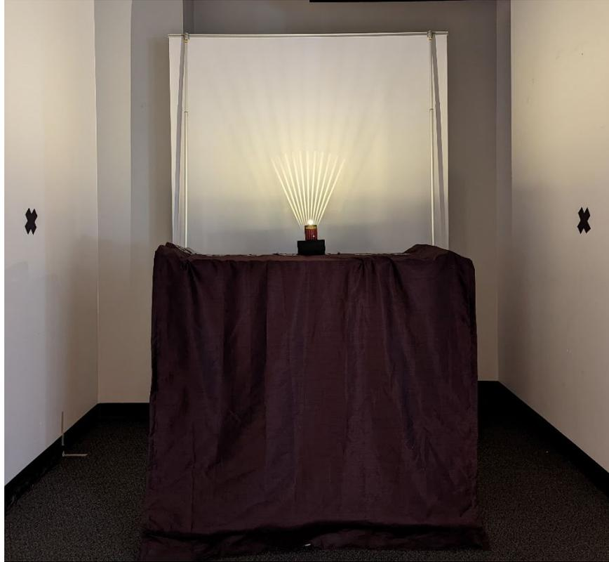
**Figure 5. Photo showing the visibility of the stroboscopic effect from the rotating wand from a high-modulation light source.**
