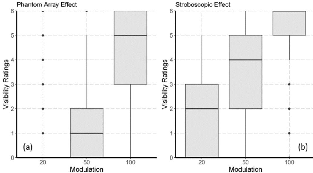
**Figure 13 (a, b).** Box plot of visibility rating medians and quartiles of 20%, 50%, and 100% modulation from rectangular TLM waveforms, phantom array (a) and stroboscopic effect (b). The phantom array effect visibility responses for 20% modulation collapsed to zero, so no box or whiskers are visible.
