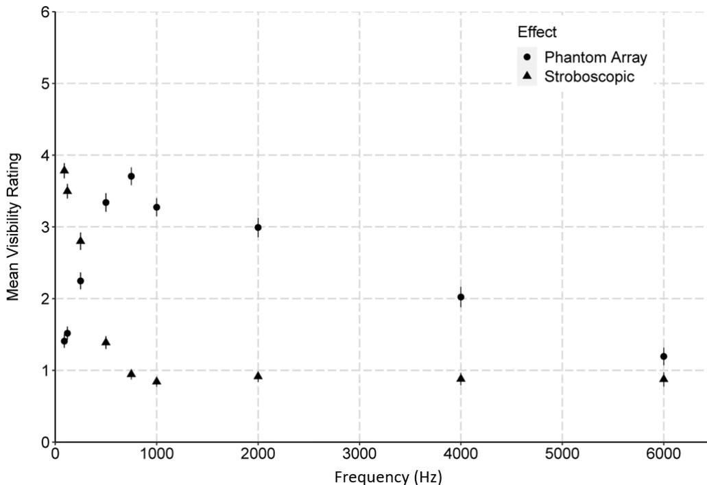
**Figure 11. Mean visibility ratings and standard error (vertical bars) for the phantom array and stroboscopic effects, combining all TLM waveforms for each effect by frequency.**
