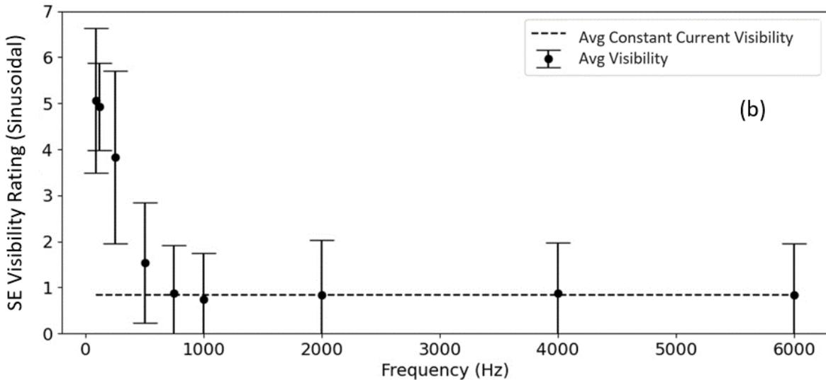
**Figure 10 (a, b): Plot of arithmetic average stroboscopic effect visibility ratings with standard deviation by frequency for two families of 100% modulation waveforms: rectangular with 30% duty cycle (a), and sinusoidal (b).**
