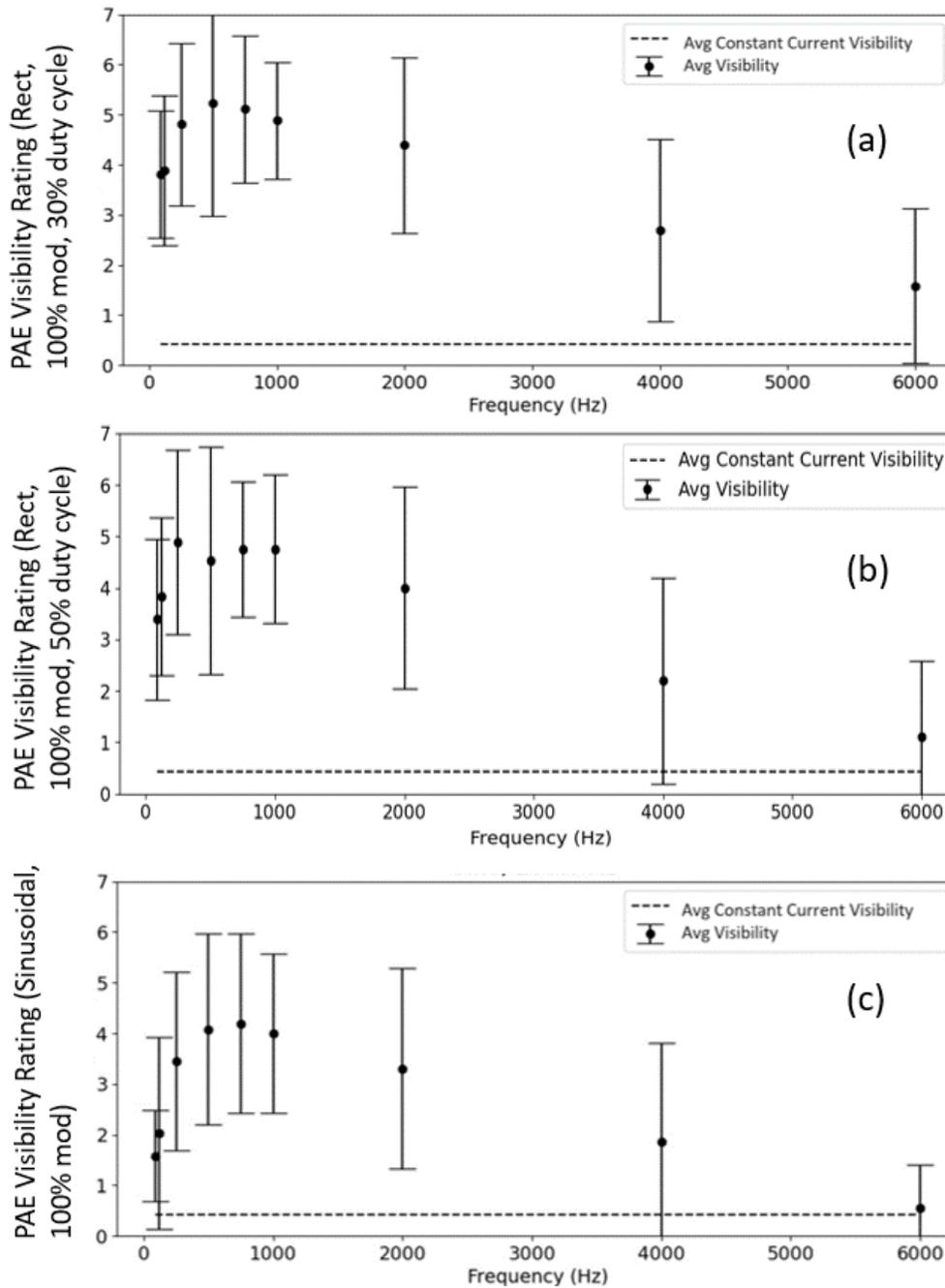
Figure 8 (a, b, c): Plots of arithmetic average phantom array effect visibility ratings with standard deviation by frequency for two families of 100% modulation waveforms: rectangular with 30% duty cycle (a), rectangular with 50% duty cycle (b), and sinusoidal (c).
