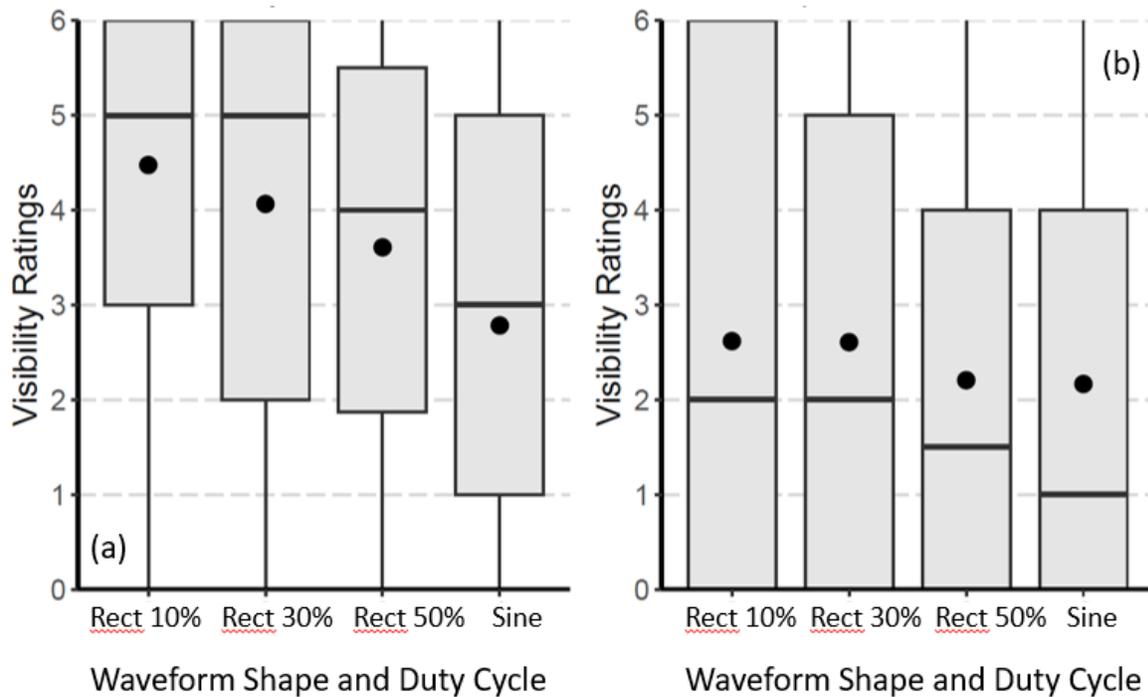
**Figure 12 (a, b).** Box plots with medians and quartiles of the visibility ratings of rectangular waveforms at three duty cycles, versus sinusoidal TLM waveforms at the same frequency and % modulation. (a) is the phantom array effect; (b) is the stroboscopic effect. Although the data set is not normally distributed, dots representing approximate arithmetic means are shown for reference.
