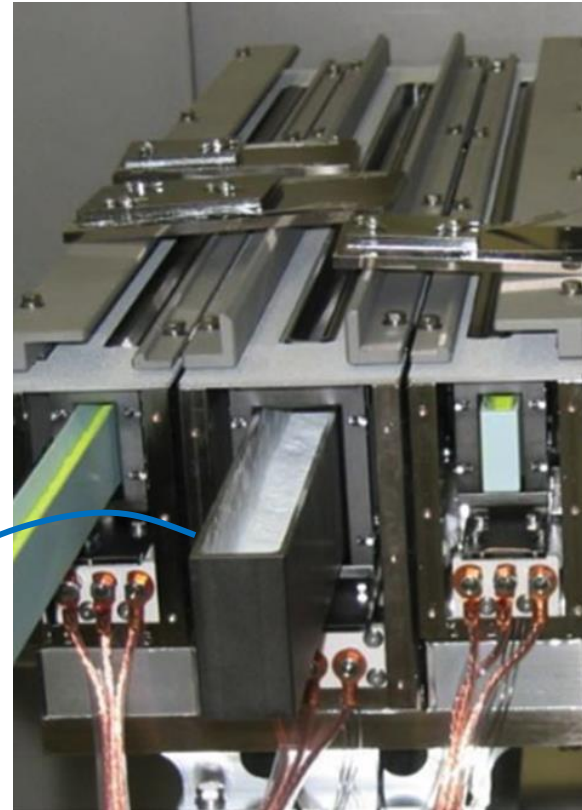
ITO-coated high aspect ratio OW substrate ready for deposition
