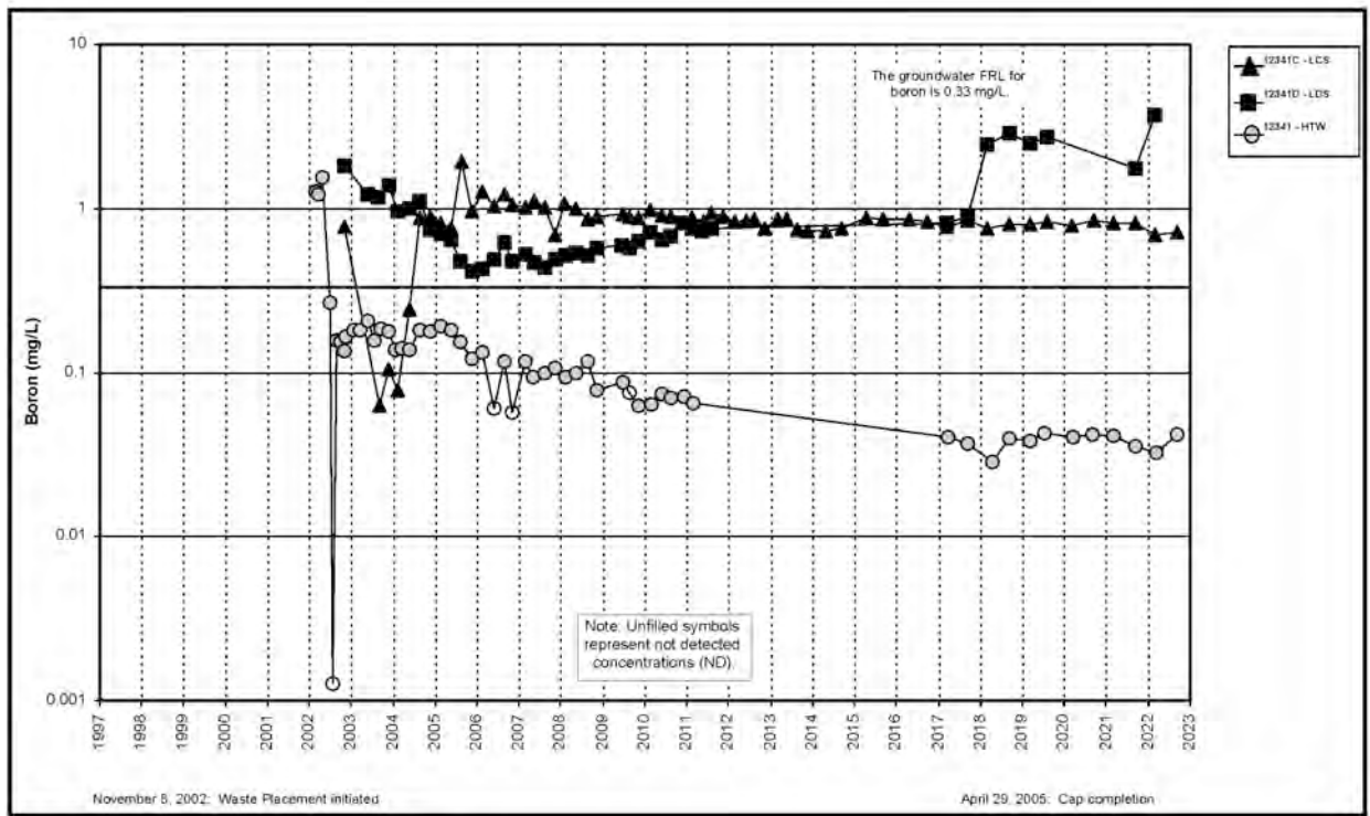
Figure A.5.4-6A. Cell 4 Boron Concentration Versus Time Plot for LCS, LDS, and HTW
