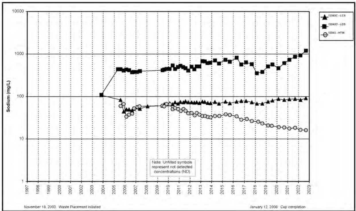
Figure A.5.6-7A. Cell 6 Sodium Concentration Versus Time Plot for LCS, LDS, and HTW
