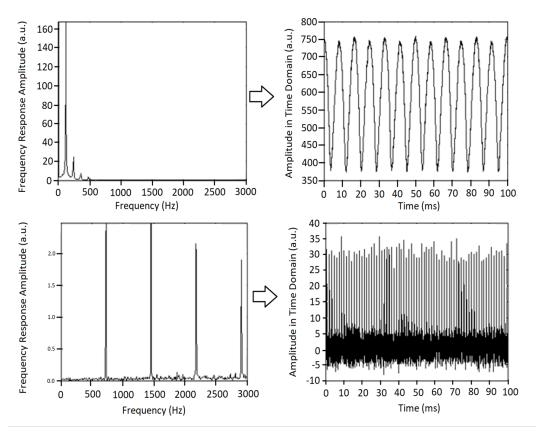
Figure 4. Two TLM waveforms plotted in the frequency domain (left) and the time domain (right).
