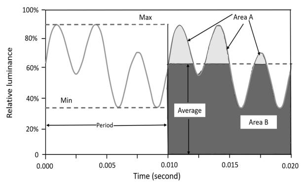
Figure 5. A periodic TLM waveform illustrating period, frequency, and values critical for calculating percent flicker and flicker index.
