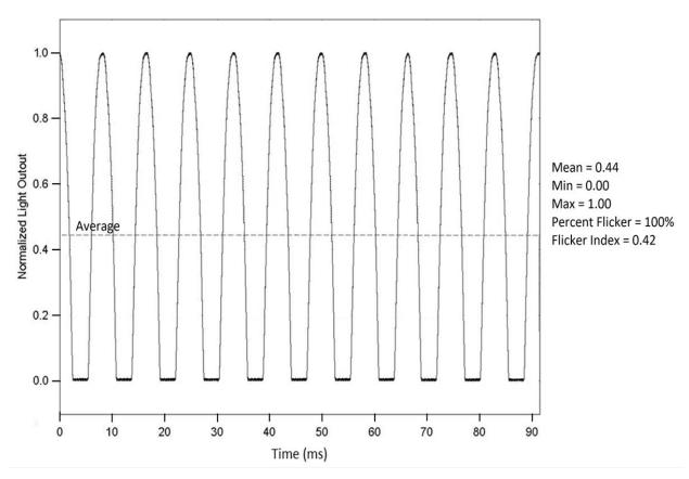
Figure 3. Waveform for an early AC-LED source, producing 120 Hz modulation. (Source: PNNL)
