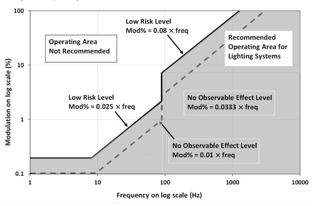
Figure 11. IEEE 1789-2015 recommended operating area to reduce visual discomfort, annoyance, and health effects of modulating light. Combinations of Percent Flicker (Modulation (%)) and fundamental frequency at the Low-Risk and No Observable Effects Levels fall in the shaded area. (Figure adapted from IEEE 1789-2015.)
