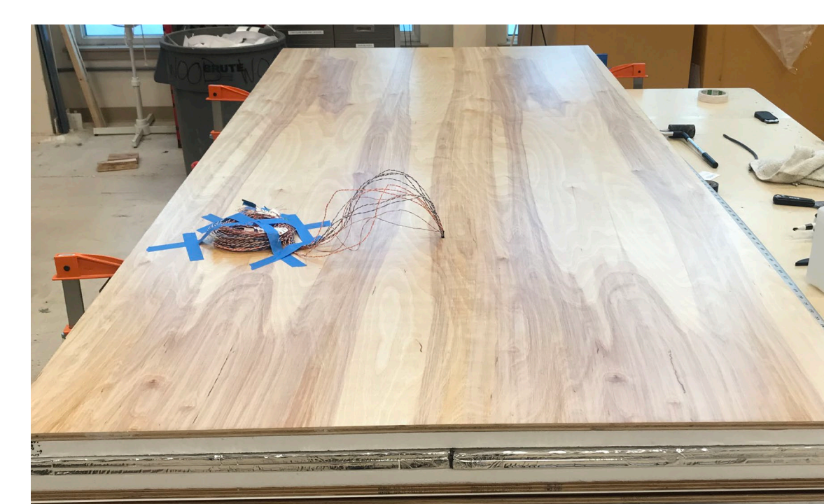
The structural frame is made with standard glulam lumber, each 4' x 8'. Adaptable composite panel has four 1-in. thick 2' x 4' fiberglass-core VIPs, and the basic building system provides aesthetics. Photos by Stacey Fritz, NREL
