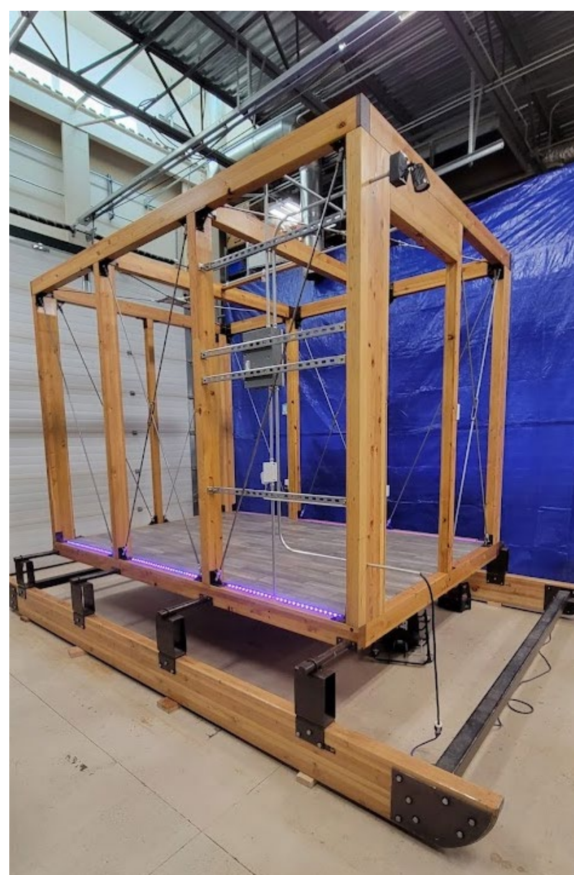
The structural frame is made with standard glulam lumber, each 4' x 8'. Adaptable composite panel has four 1-in. thick 2' x 4' fiberglass-core VIPs, and the basic building system provides aesthetics. Photos by Stacey Fritz, NREL
