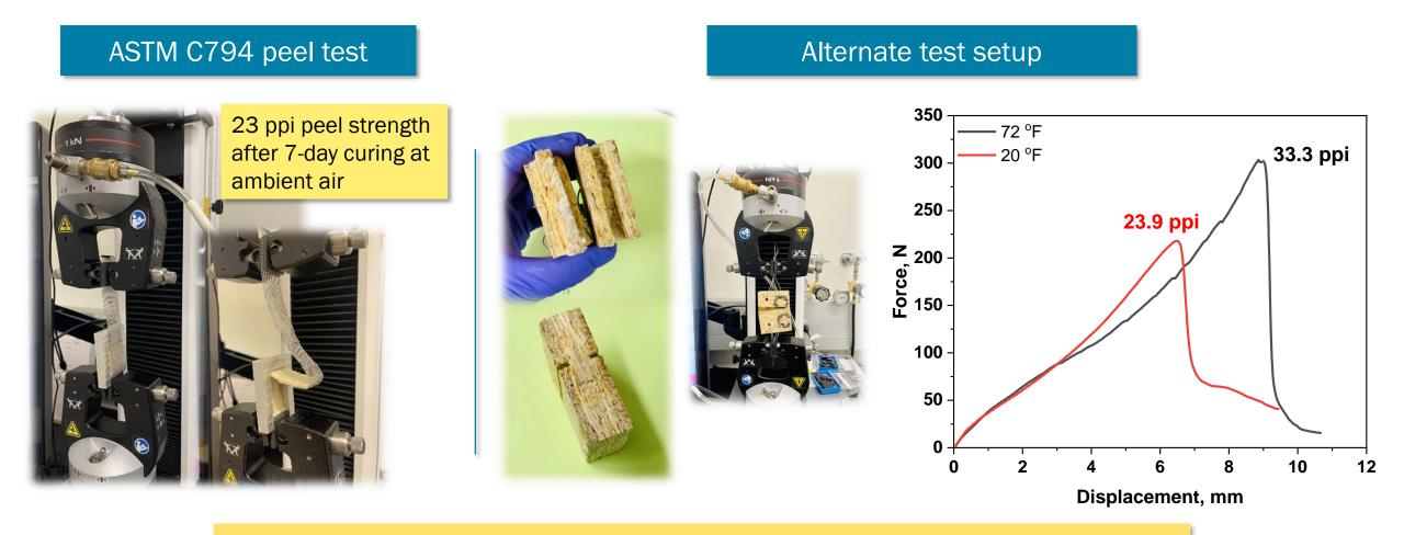
Nonoptimized epoxy-based formulation exceeded 20 ppi peel strength target after curing at ambient and 20°F for 21 days
