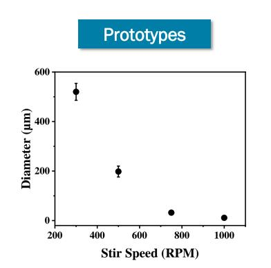
Demonstrated encapsulation of iso- and epoxy-based reactive agents with tunable diameters
