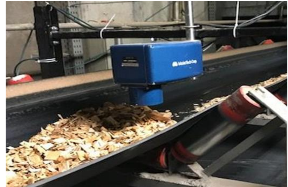
MoistTech: Non-contact moisture sensors appropriate for use in a continuous process
