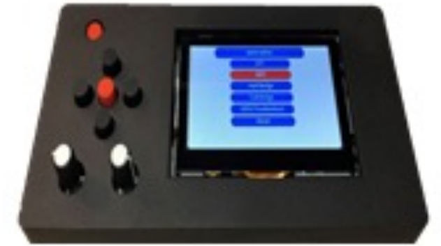
Fig. 8 UAC-106 general purpose controller platform
