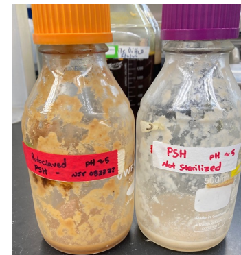
Residual Solids After (left) and Before (right) autoclaving Pea Starch Hydrolysate
