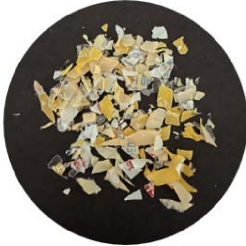
Shredded post-industrial multilayer printed plastic film
