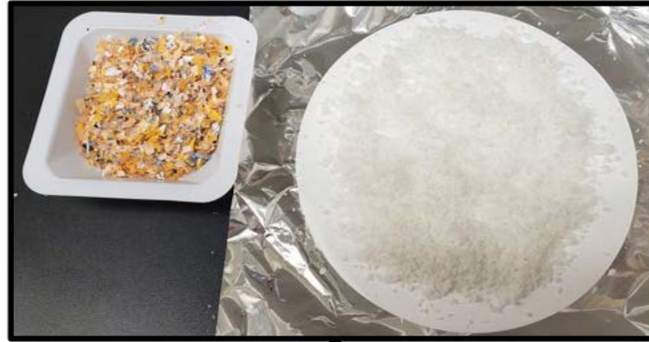
Recovery of PE component from printed film via STRAP
