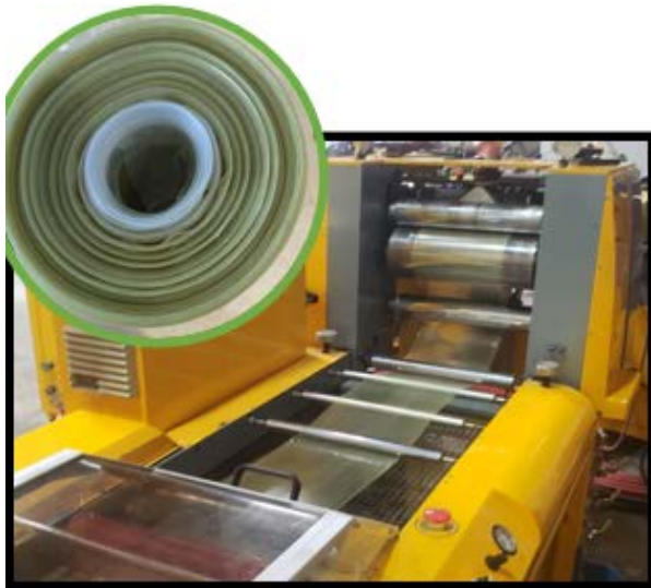
Production of 100% recycled PE film
