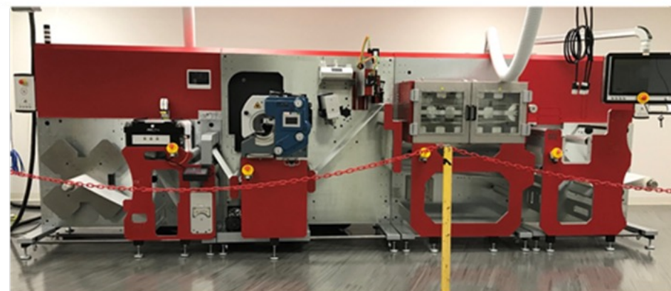
Roll-to-roll screen printing and slot-die coating- Pilot-scale continuous membrane synthesis
