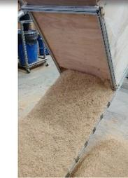
— (INL) Inclined plane flow tester
