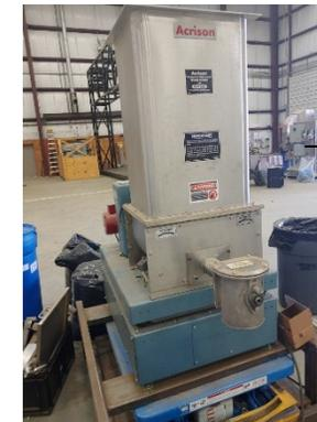
— (INL) Screw feeder for testing mechanically driven flow
