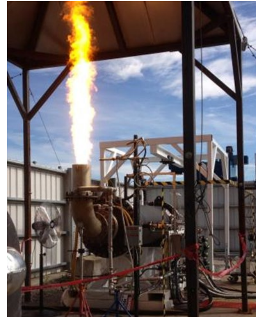
Linde pilot-scale HOB Connected to LanzaTech mobile pilot plant
