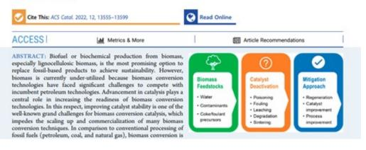
Connection between biomass feedstocks and catalysts with potential catalyst deactivation and mitigation
