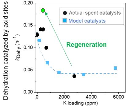
A study of the real spent Pt/TiO<sub>2</sub> catalysts validates the impact of K and the regeneration developed based on the model system
