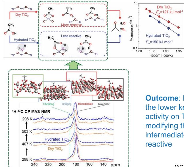
**Outcome**:  $H_2O$  leads to the lower ketonization activity on  $TiO_2$  by modifying the surface intermediates to be less reactive
