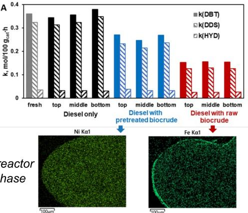
**Outcome**: The results suggest the need of 1) bio-crude pretreatment; and 2) guard bed improvement to enable minimal impact on hydrotreating catalyst stability when co-processing bio-crude
