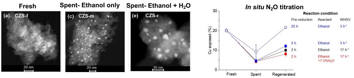
Greater sintering of Cu observed for ethanol/water than ethanol only feed
