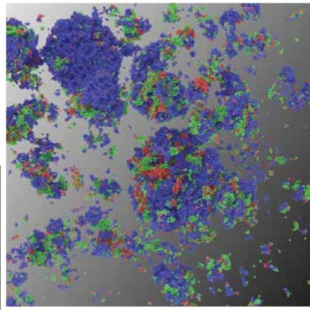
➤ Molecular dynamics models simulate collections of atoms to expose phase transitions, such as the freezing of liquid metals in extreme conditions. (LLNL)
