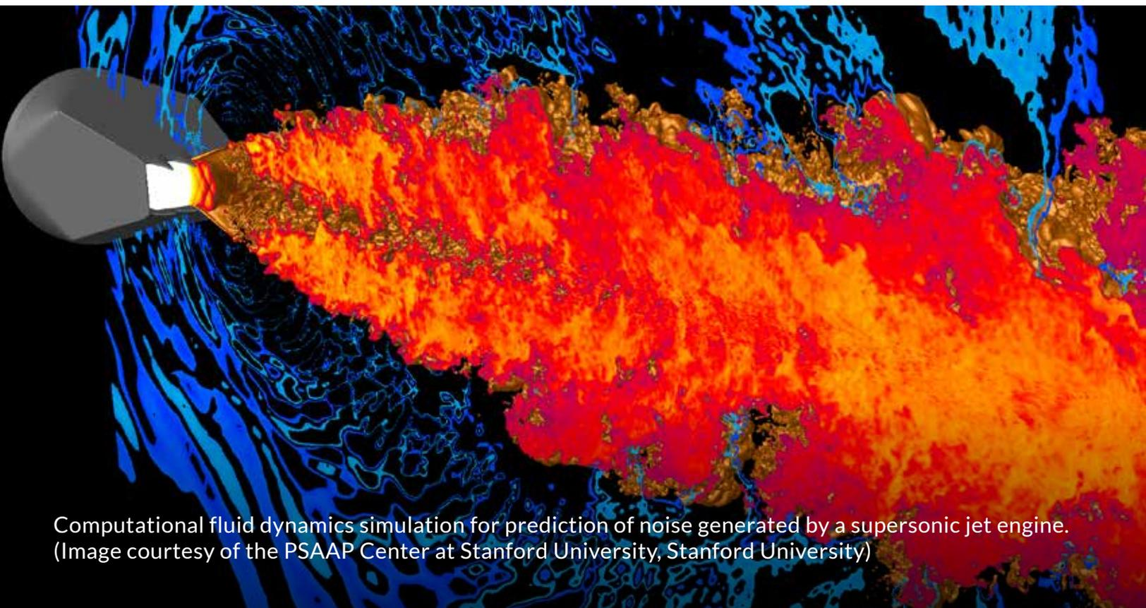
Computational fluid dynamics simulation for prediction of noise generated by a supersonic jet engine. (Image courtesy of the PSAAP Center at Stanford University, Stanford University)
