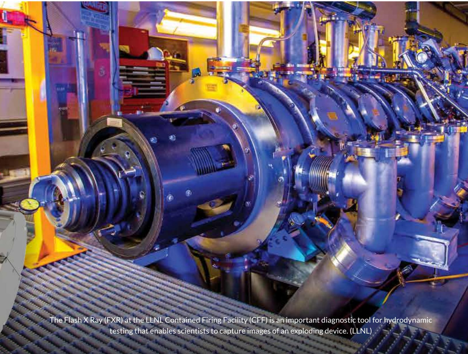
The Flash X Ray (FXR) at the LLNL Contained Firing Facility (CFF) is an important diagnostic tool for hydrodynamic testing that enables scientists to capture images of an exploding device. (LLNL)
