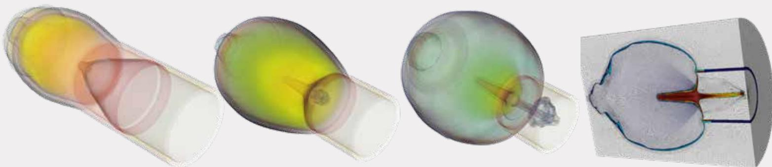
➤ The evolution of a shaped charge jet as simulated by MARBL.
