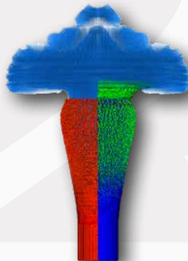
Simulation showing the explosively driven fragmentation of an AerMet steel cylinder at 25 microsec, with an image of the actual experiment for comparison. In the experiment, the high explosive is lighted at the top of the cylinder, and the burn front travels downward, expanding the explosive outward and fracturing the cylinder. In the simulation, the left side (red) shows the mass density of the intact material, while the right (green) shows the material damage.
