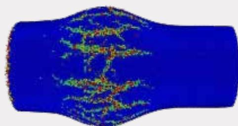
➤ The comparison between an image of an explosively driven cylinder and a simulation using the SPH method.
