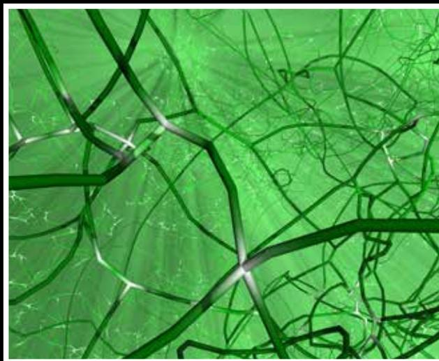
➤ A dislocation multijunction discovered in a ParaDiS (LLNL) dislocation dynamics simulation. These simulations provide insight into how materials fail when put under stress.
