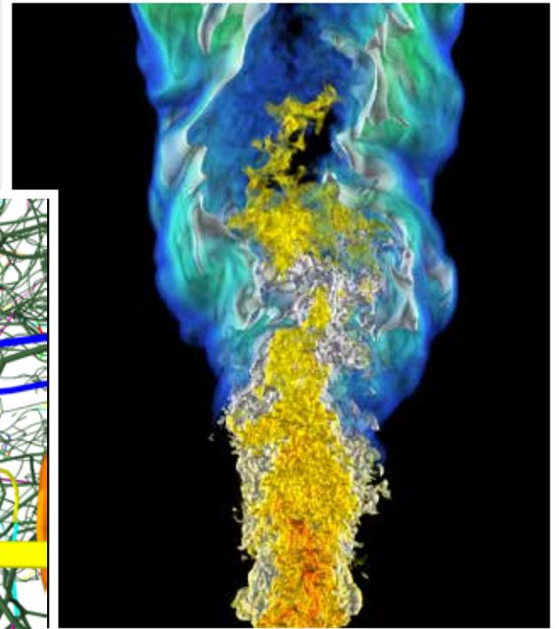
Direct numerical simulation reveals turbulent combustion of a lifted ethylene/air jet flame in a heated coflow of air. (SNL)
