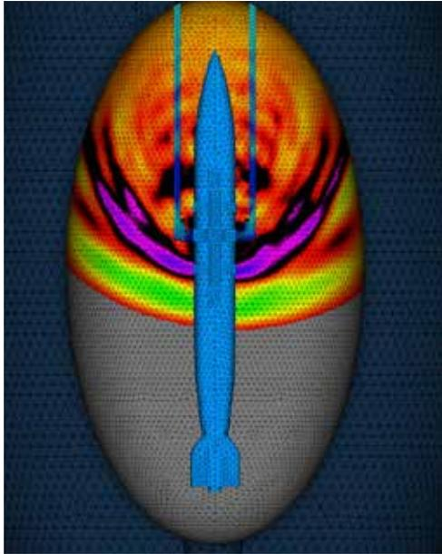
Simulation using the structural dynamics (SD) component of the SIERRA multiphysics code, depicting structural response for the B61-12 to acoustic loading. (SNL)
