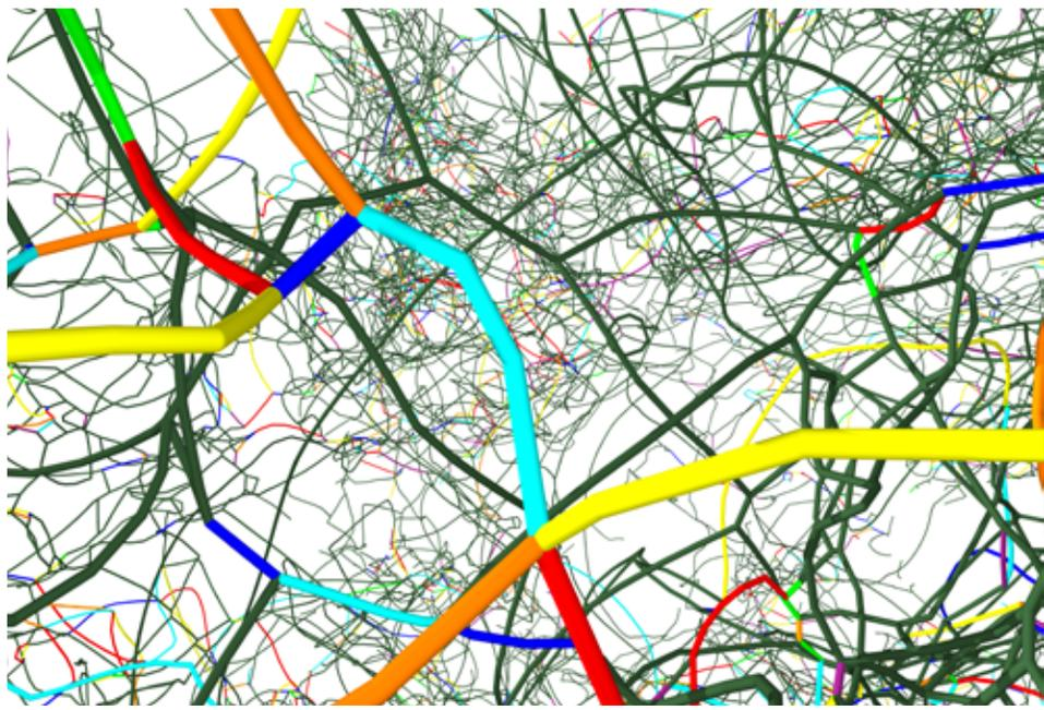
Rendering of a dislocation multijunction discovered in a ParaDiS dislocation dynamics simulation. Multijunctions are new topological dislocation configurations discovered through simulation that are key to understanding the hardening of body centered cubic alloys. (LLNL)
