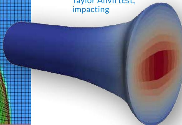
Comparing deformation in the simulated cylinder against results of a live experiment enables validation of the hydrodynamic algorithms used in the simulation (Hungerford, 2021; Zecevic, 2021).
