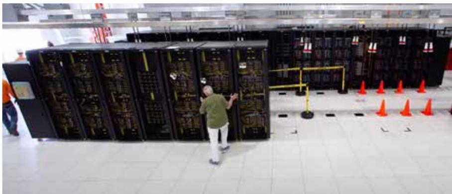
Technicians build the Attaway (CTS-1) supercomputer from Penguin Computing at SNL.
