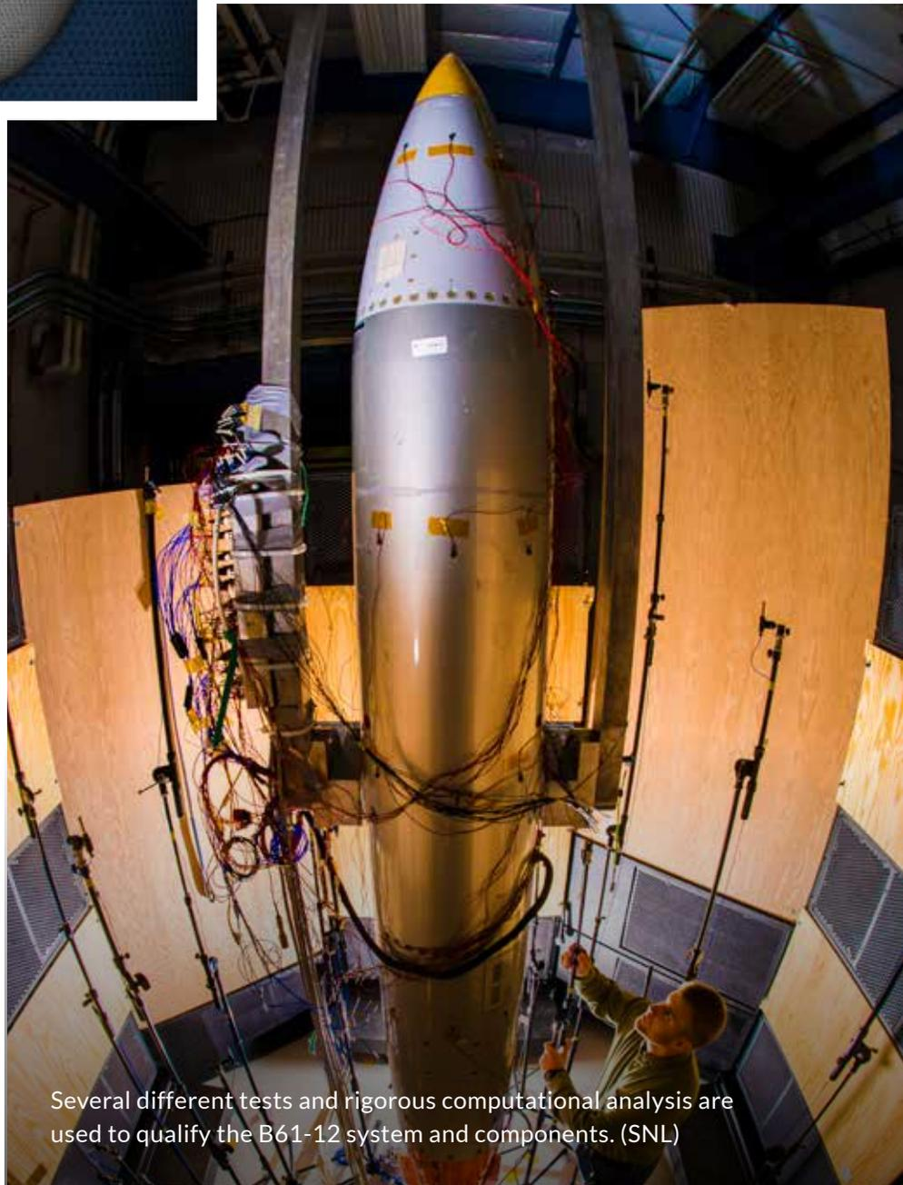
Several different tests and rigorous computational analysis are used to qualify the B61-12 system and components. (SNL)
