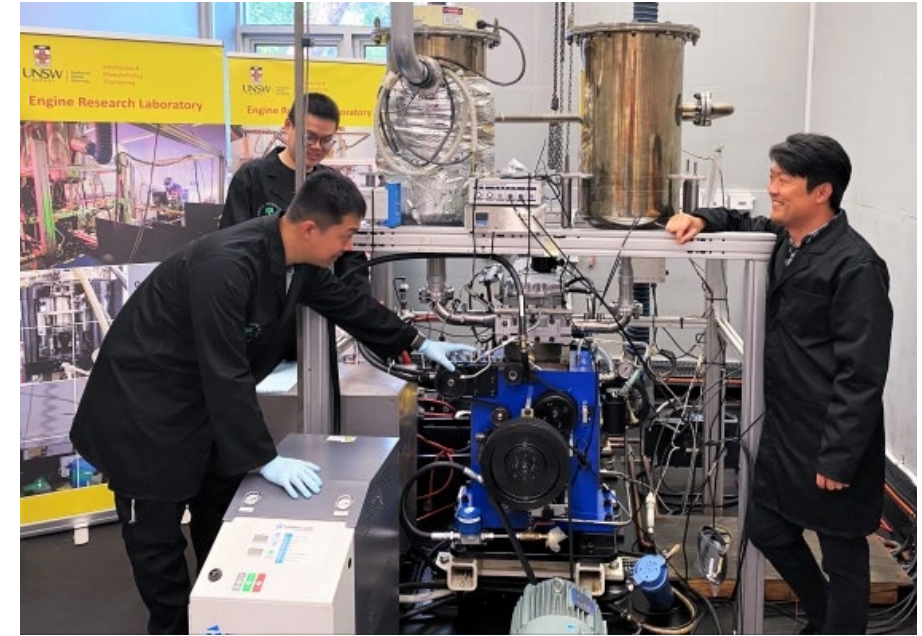
H 2 -diesel dual-fuel single cylinder engine
