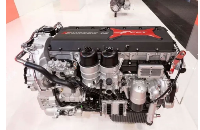
FPT XC13 13L multi-fuel engine
