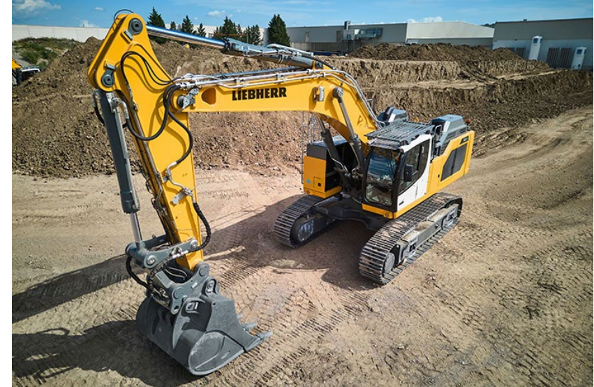
Liebherr 9XX H2 50ton excavator
