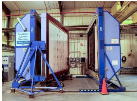
ORNL Guarded Hot Box
