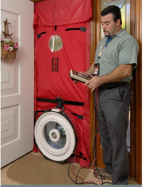
A blower door test helps evaluate a home's air tightness and is an important part of the initial assessment.
