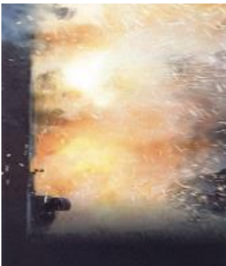
Figure 2-7. This photo shows the energy released from thermal, pressure, sound, and light modes during a typical arc-flash event.
