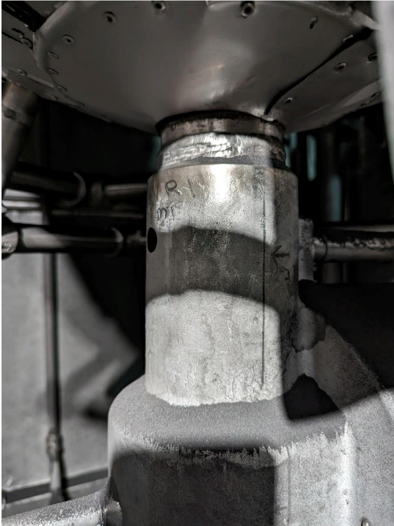
Eroded hole below PRC-0
