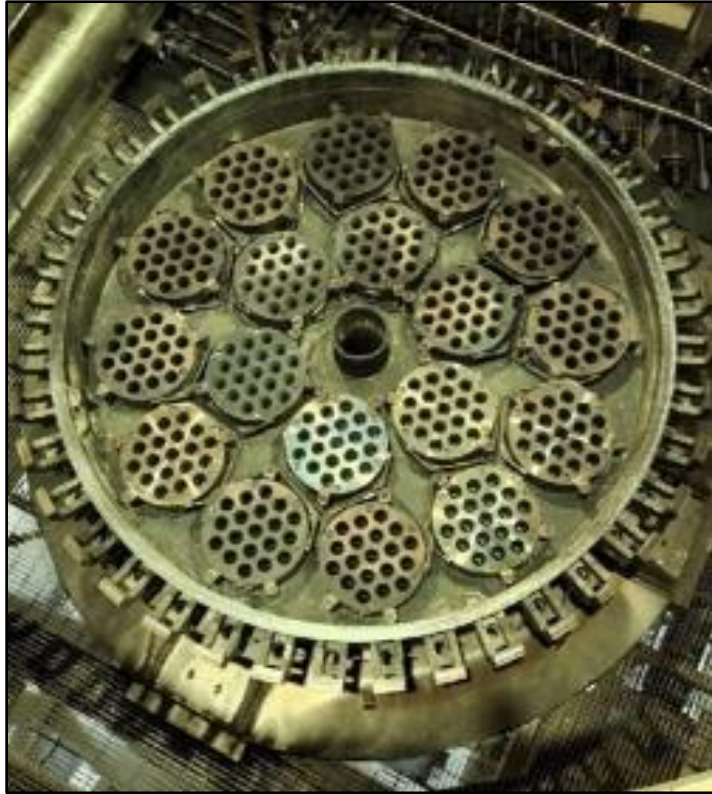
PGF tubesheet and filter inspection following confirmatory run
