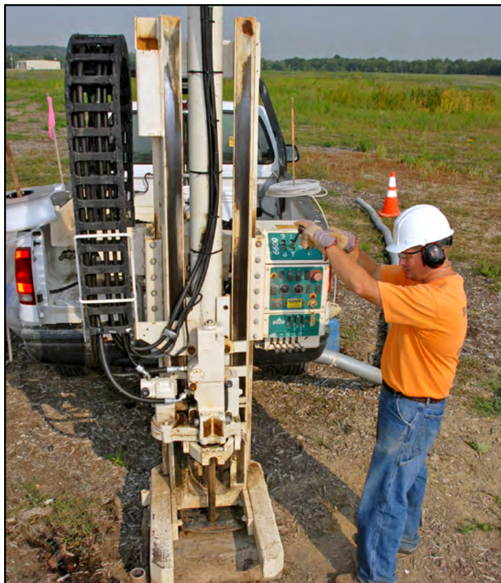
Typical equipment (pickup truck with drill rig attachment known as a Geoprobe rig) used for collecting soil gas samples at the Mound site.
