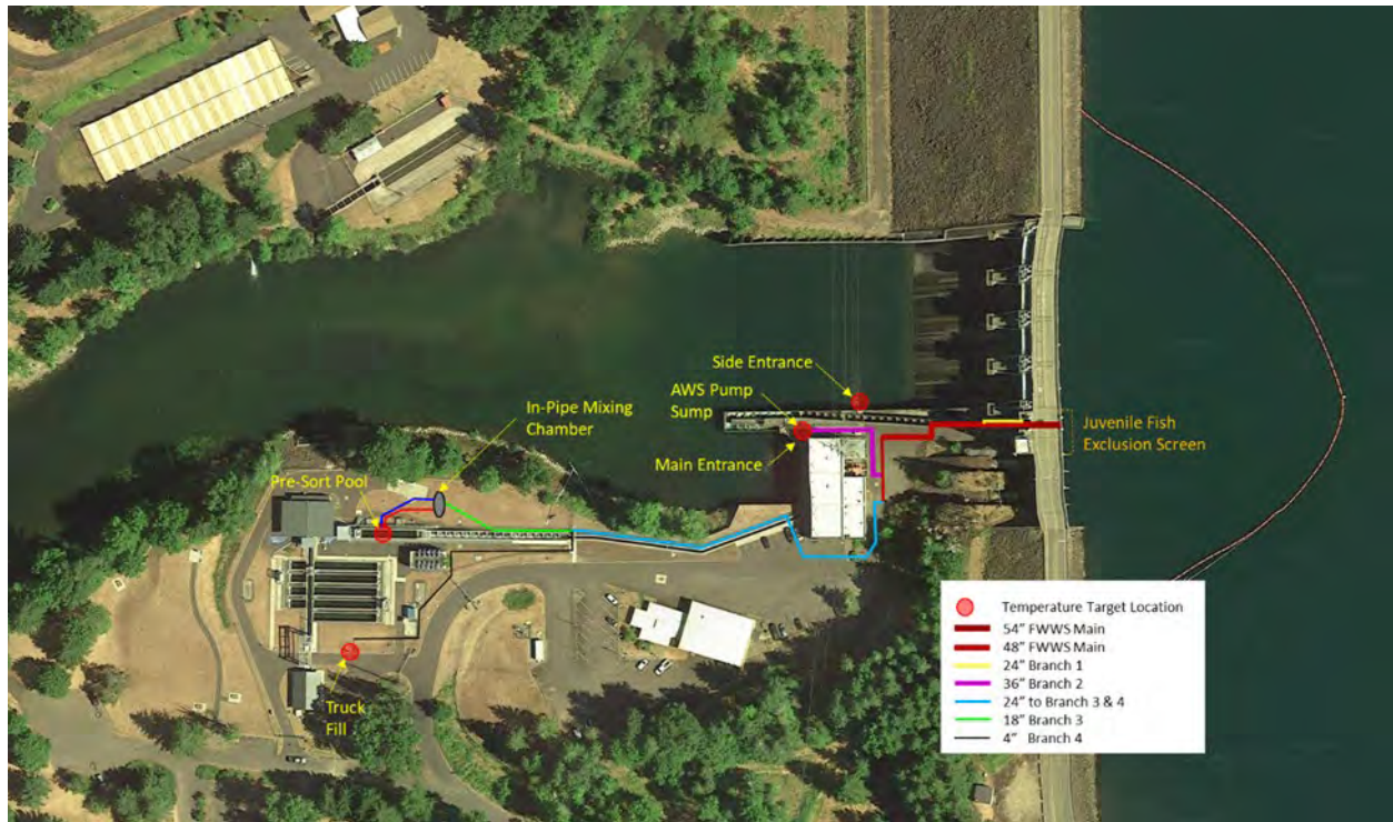
Figure 2.2-6. FWWS Piping Schematic with Temperature Target Locations (at Foster Dam)
