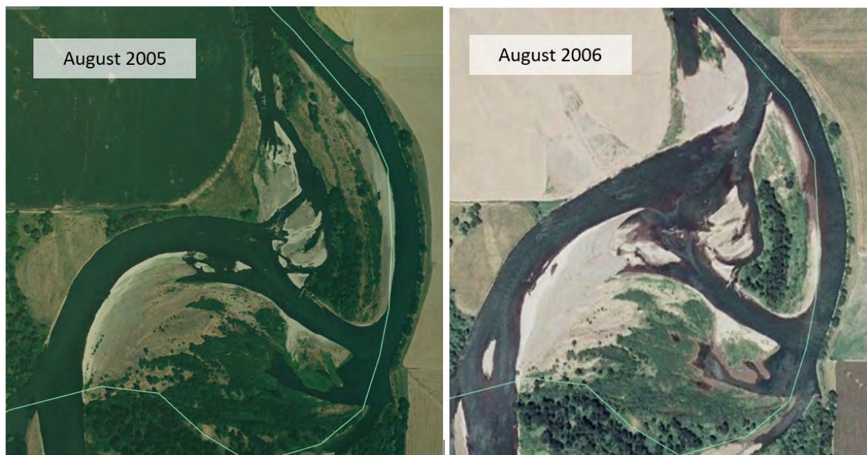
Figure 3.3-7. Willamette River realignment before and after January 2006 flood, south of Peoria, OR
