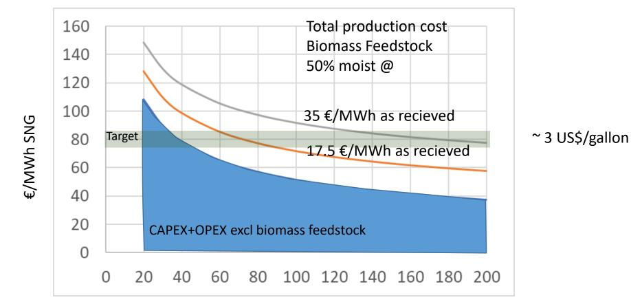
Plant size MW SNG 100 MW correspond to around 60 000 ton SNG/year 25 fully loaded trucks with biomass a day
