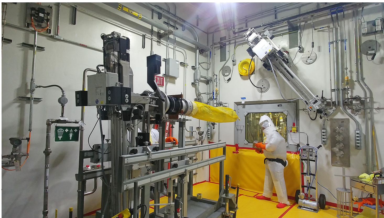
The SWPF laboratory uses manipulators to handle process samples and equipment within its radioactive cell, which help protect workers handling the radioactive materials
