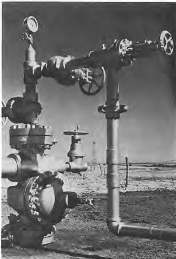
Surface control valves in a "Christmas tree" configuration, used on land or on a fixed platform over water.
